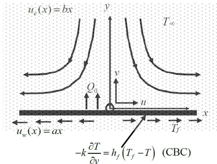
Figure 1. Physical model and the coordinate system
