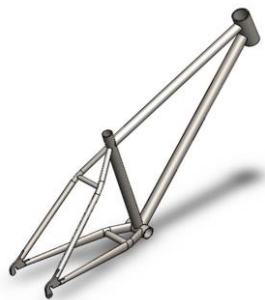
Figure 1. CAD of bicycle frame
