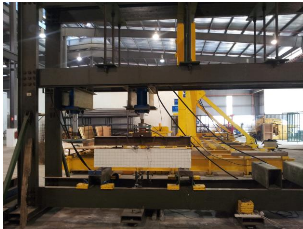
Figure 3.53: Magnus frame for four point bending test
