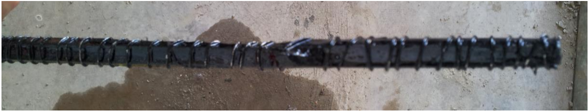
Figure 3.10: Treated bamboo stick coiled with wire
