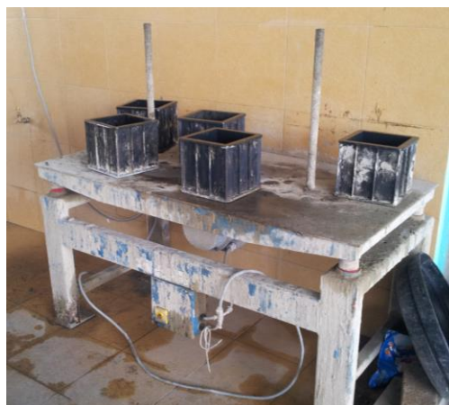
Figure 3.27: Vibrator for concrete cubes
