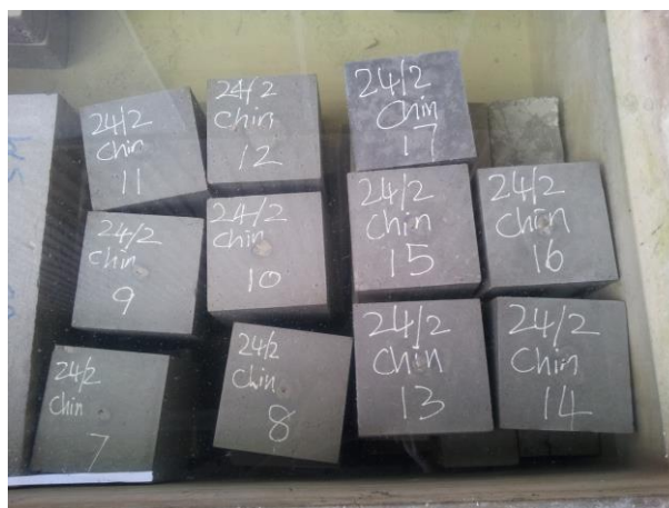
Figure 3.31: Concrete cube curing
