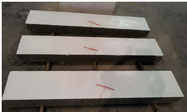
Figure 3.49: Beam specimens were painted
