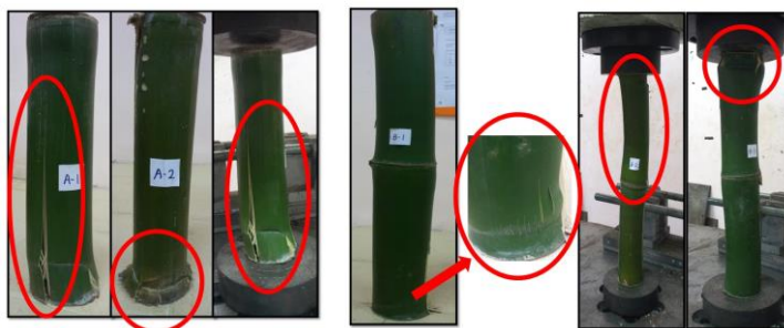
Figure 4.21: Failed bamboo samples with zero and one node
