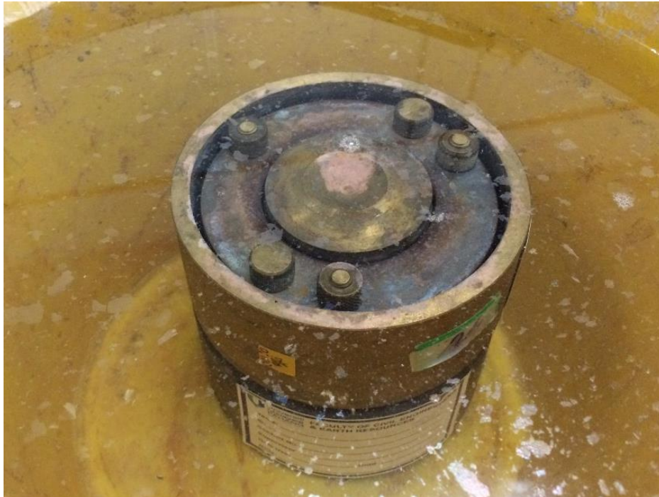
Figure 3.6: Specimen undergoes water curing process
