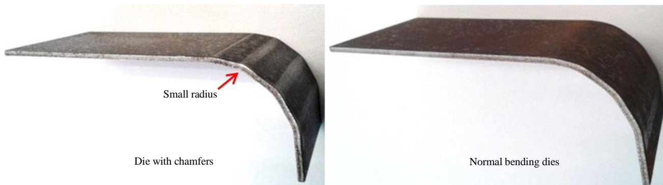
Figure 5: The bent sheets by die with chamfers and normal bending die
