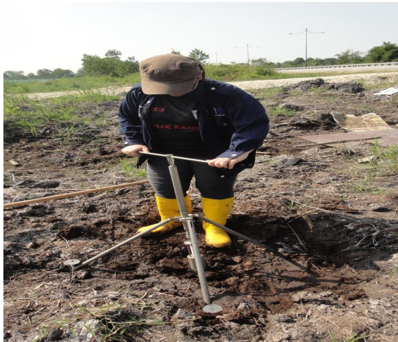
Figure 3.6 Soil sample obtained using Tropiter
