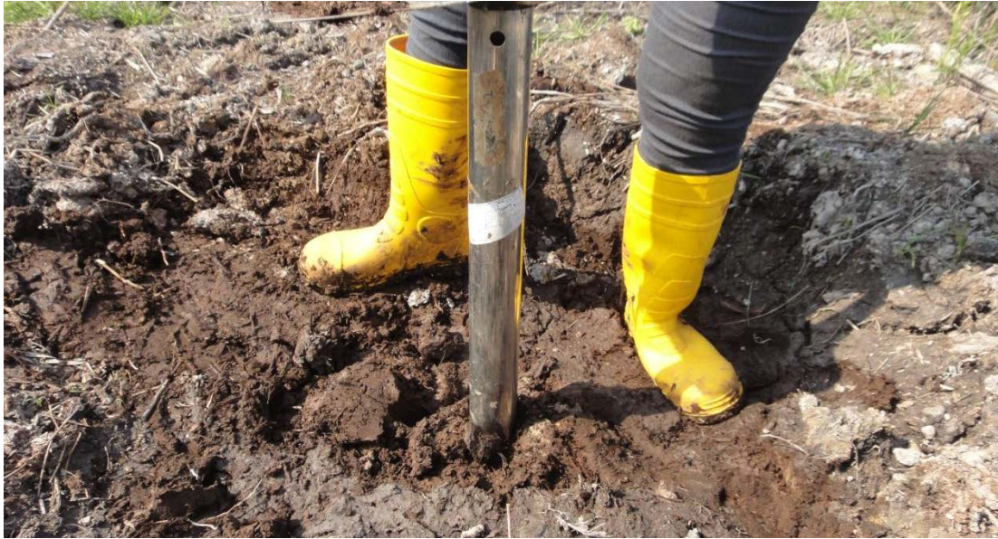
Figure 3.5 Soil sample obtained using conventional tube sampler
