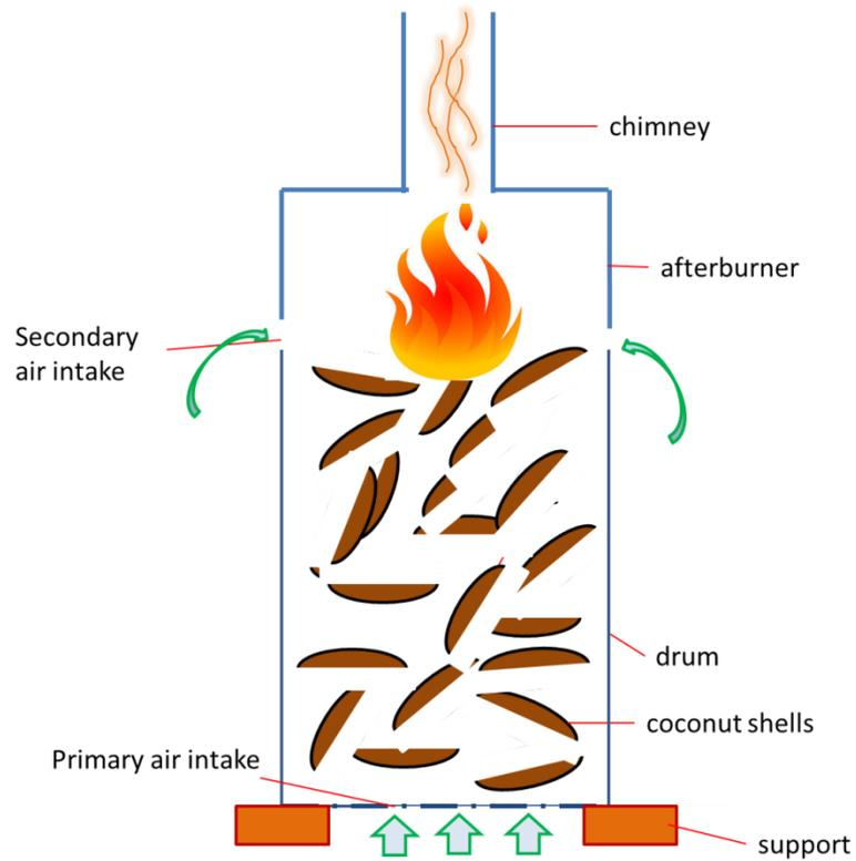
Figure 4: Schematic Top Lit Up Draft
