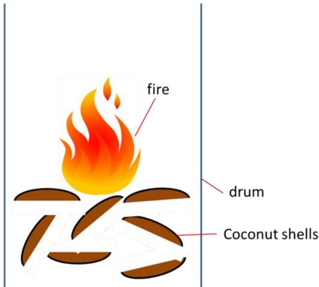
Figure 2: Schematic traditional method
