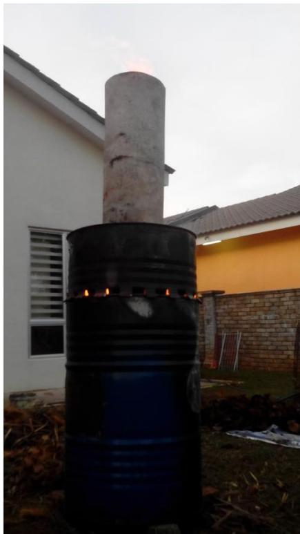
Figure 5: Picture of top Lit Up Draft Furnace
