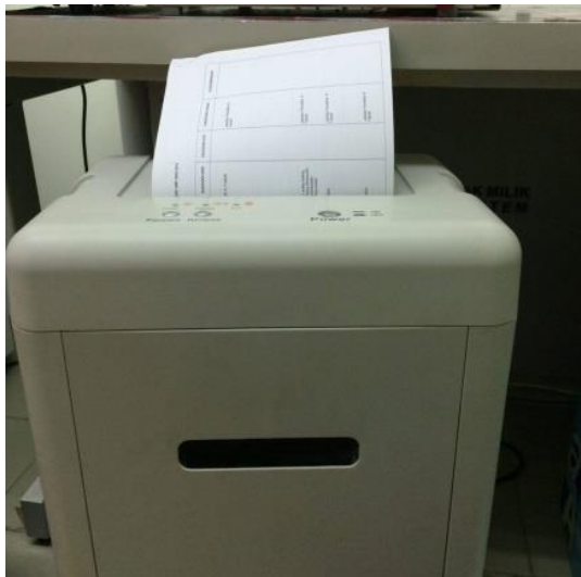
Figure 3.6: 2x8 mm Shredder machine
