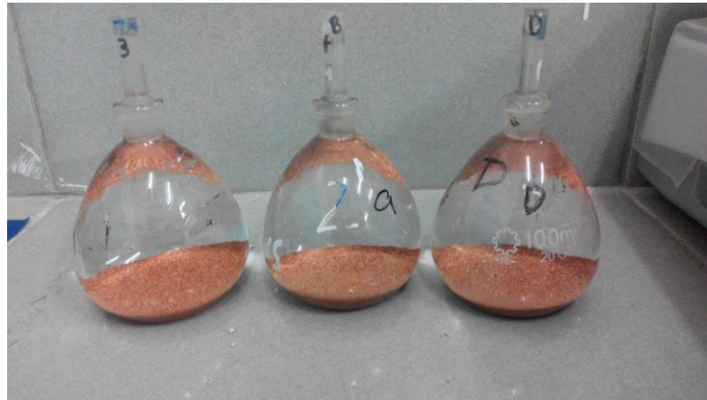
Fig. 3.1: Apparatus set-up for specific gravity test
