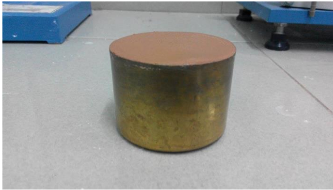
Fig. 3.2: Apparatus set-up for shrinkage limit test
