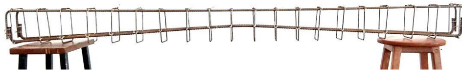
Figure 3.8: Front view reinforcement cage for Specimen 3.
