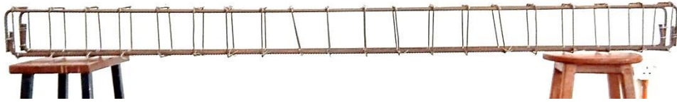
Figure 3.6: Front view of reinforcement cage for Specimen 1 (control).
