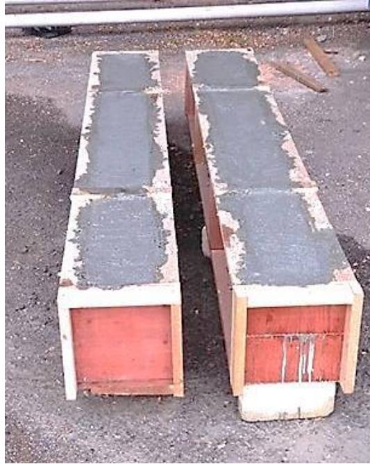
Figure 3.12: Screeding of specimens.
