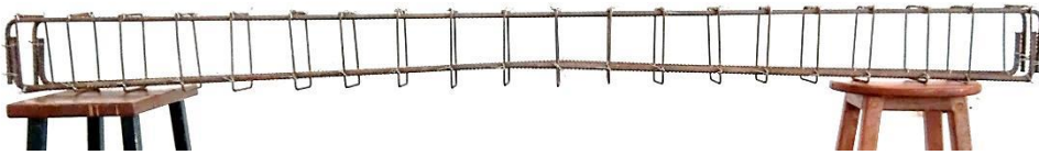
Figure 3.7: Front view reinforcement cage for Specimen 2.
