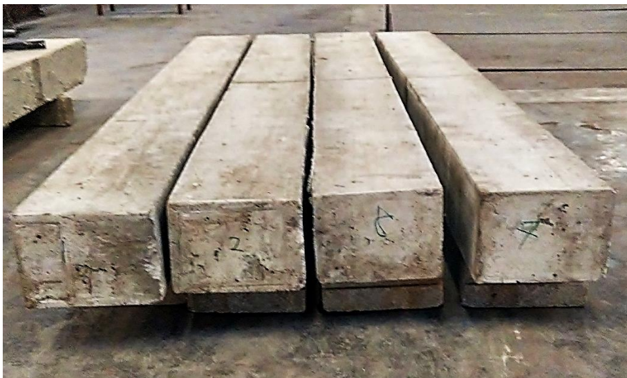
Figure 3: Reinforced concrete beam after curing process.
