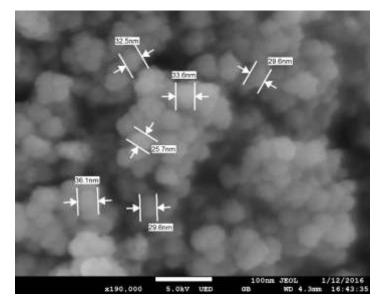
Fig. 1. SiO<sub>2</sub> nanoparticles with average size of 30 nm.
