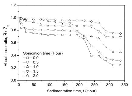
Fig. 6. Absorbance ratio of SiO<sub>2</sub>/PAG nanolubricant as a function of sedimentation time.
