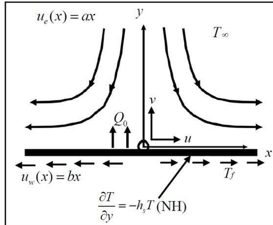
FIGURE 1. The physical model of coordinate system
