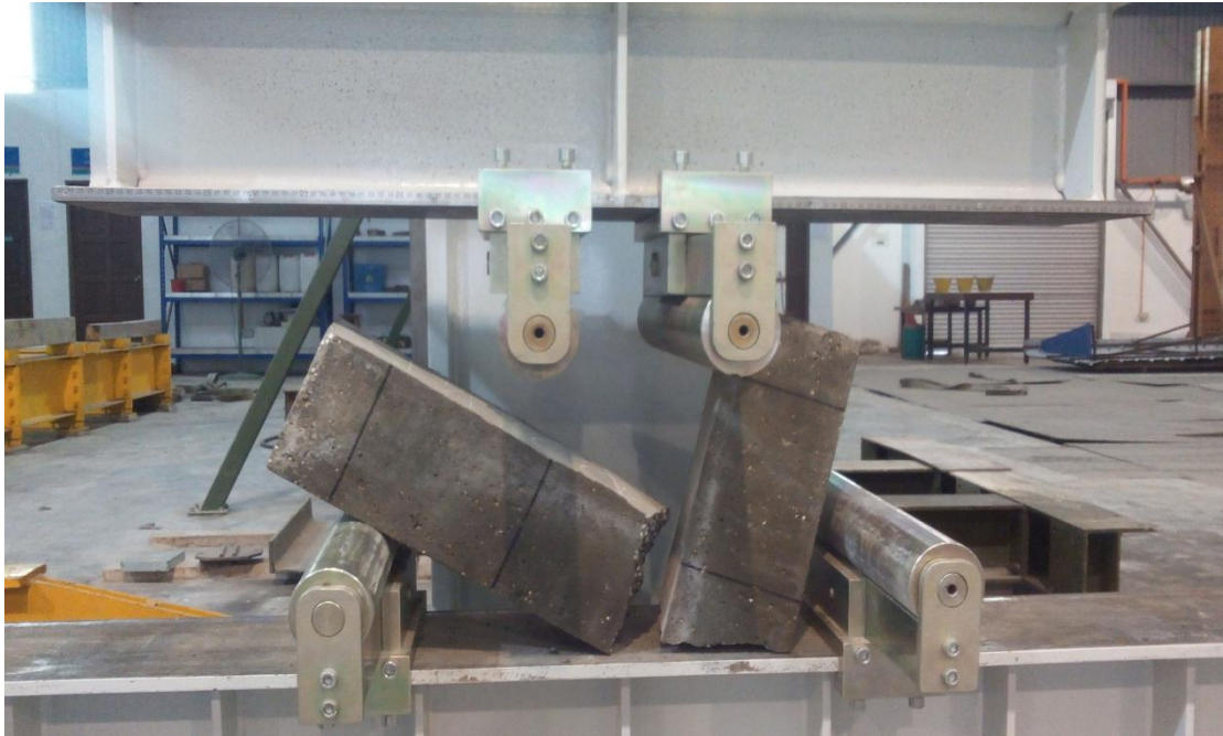
Figure 4.22: Patten of failure of beam on days 14 for ratio 2 sample
