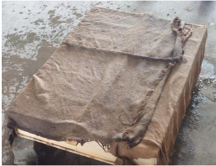
Figure 3.14: Curing process for beam sample
