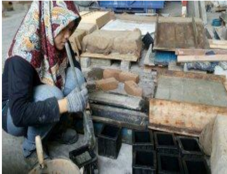
Figure 3.9: Compact the concrete using stamping rod
