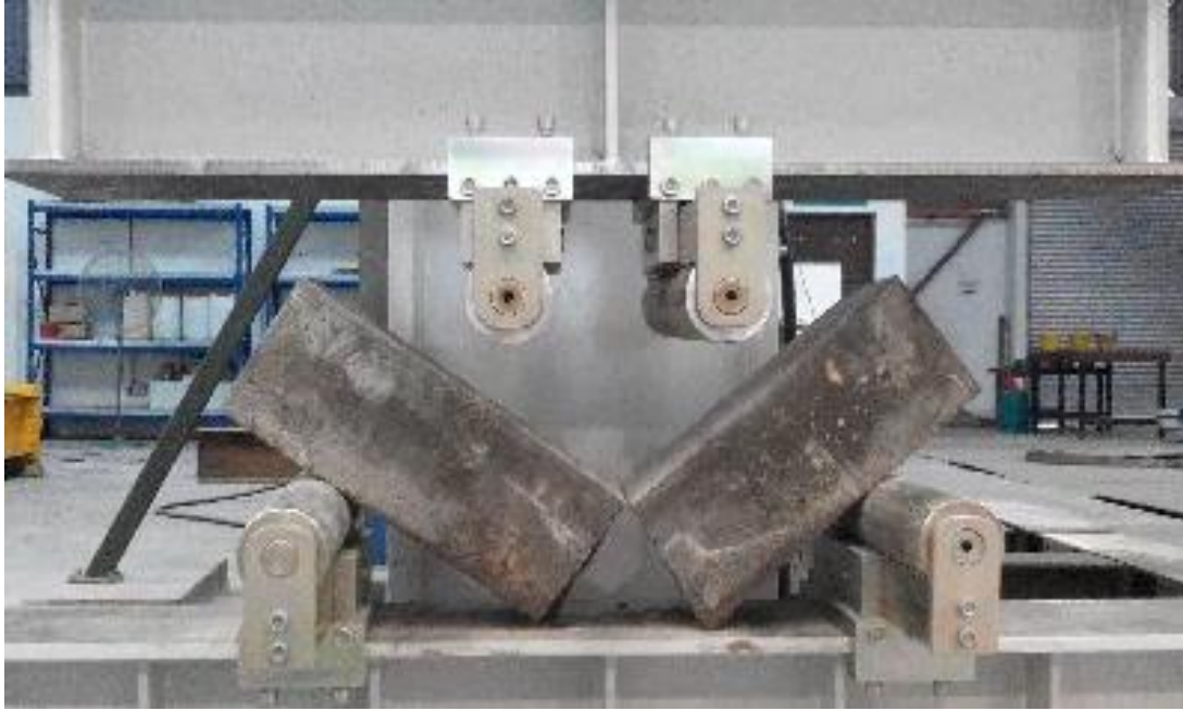
Figure 4.18: Patten of failure at 14-days for control sample
