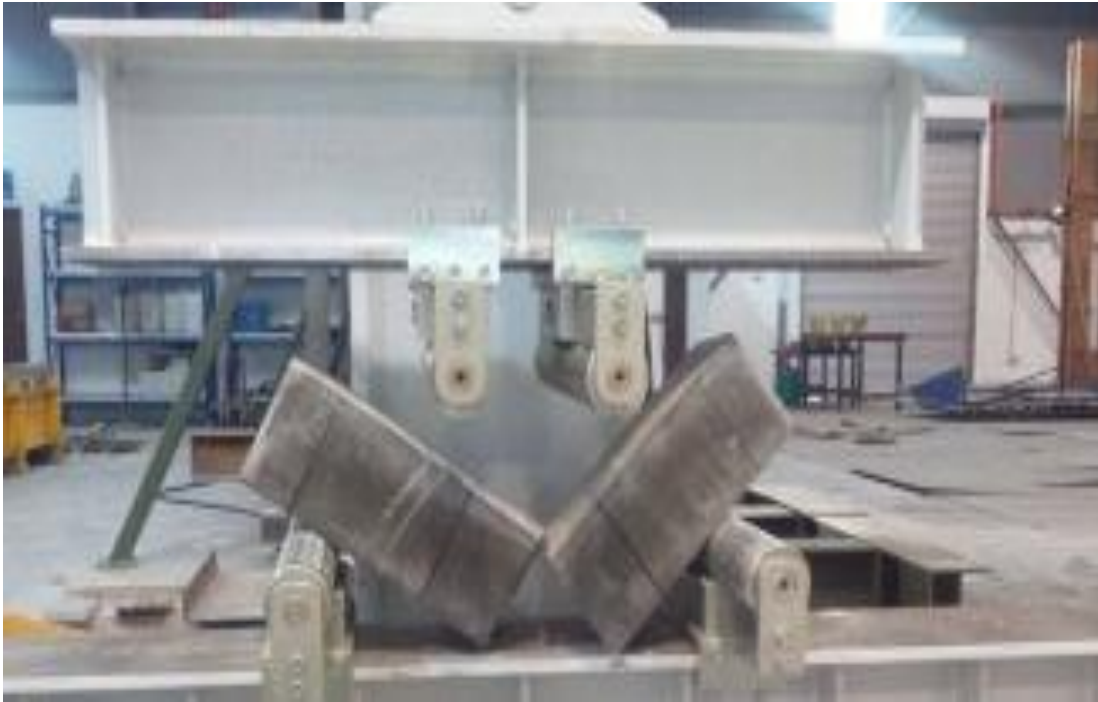
Figure 4.20: Patten of failure of beam on days 14 for ratio 1 sample
