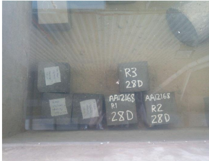
Figure 3.13: Curing process for cube sample
