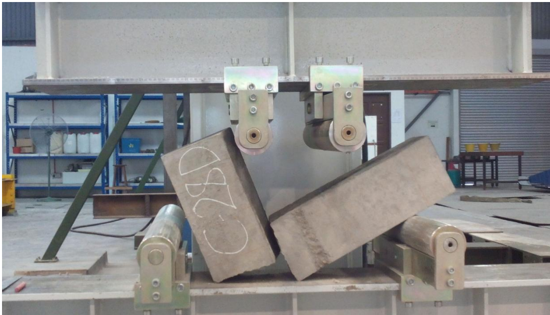
Figure 4.19: Patten of failure of beam on days 28 for control sample
