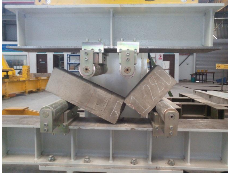
Figure 3.25: Load is stop applied when sample failed
