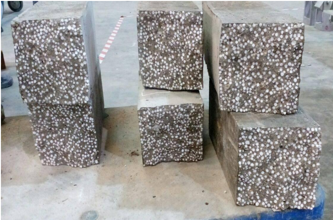
Figure 4.28: 25% of polystyrene beads in concrete for ratio 2
