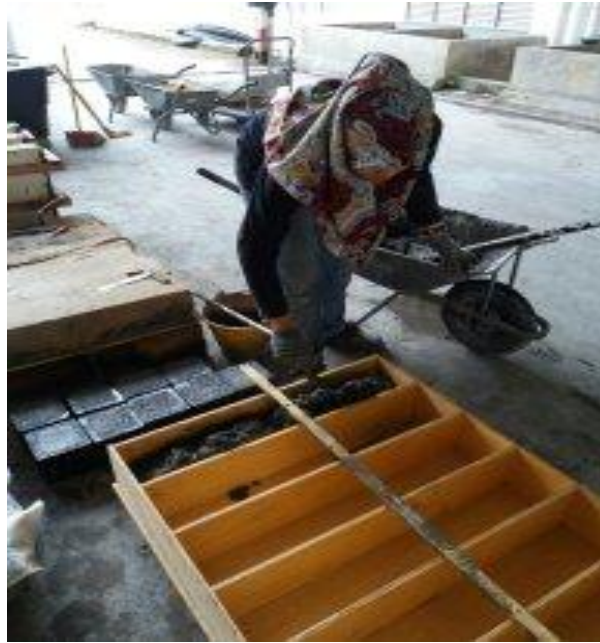
Figure 3.11: Process for making beam sample
