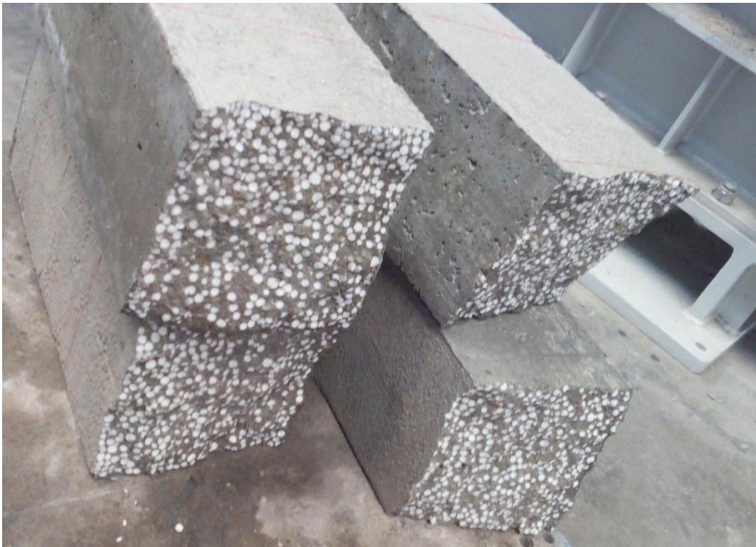
Figure 4.29: 37.5% of polystyrene beads in concrete for ratio 3
