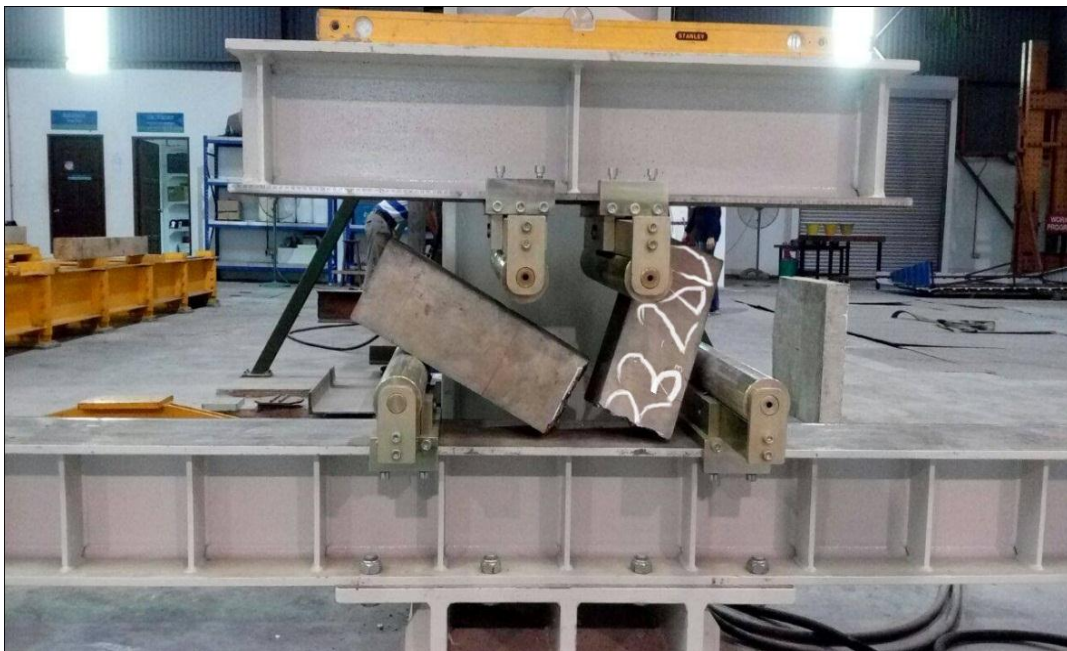
Figure 4.25: Patten of failure of beam on days 28 for ratio 3 sample
