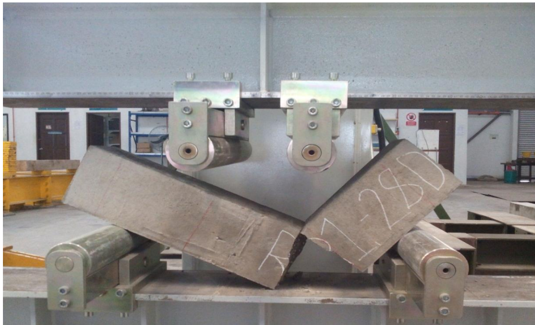
Figure 4.21: Patten of failure of beam on days 28 for ratio 1 sample
