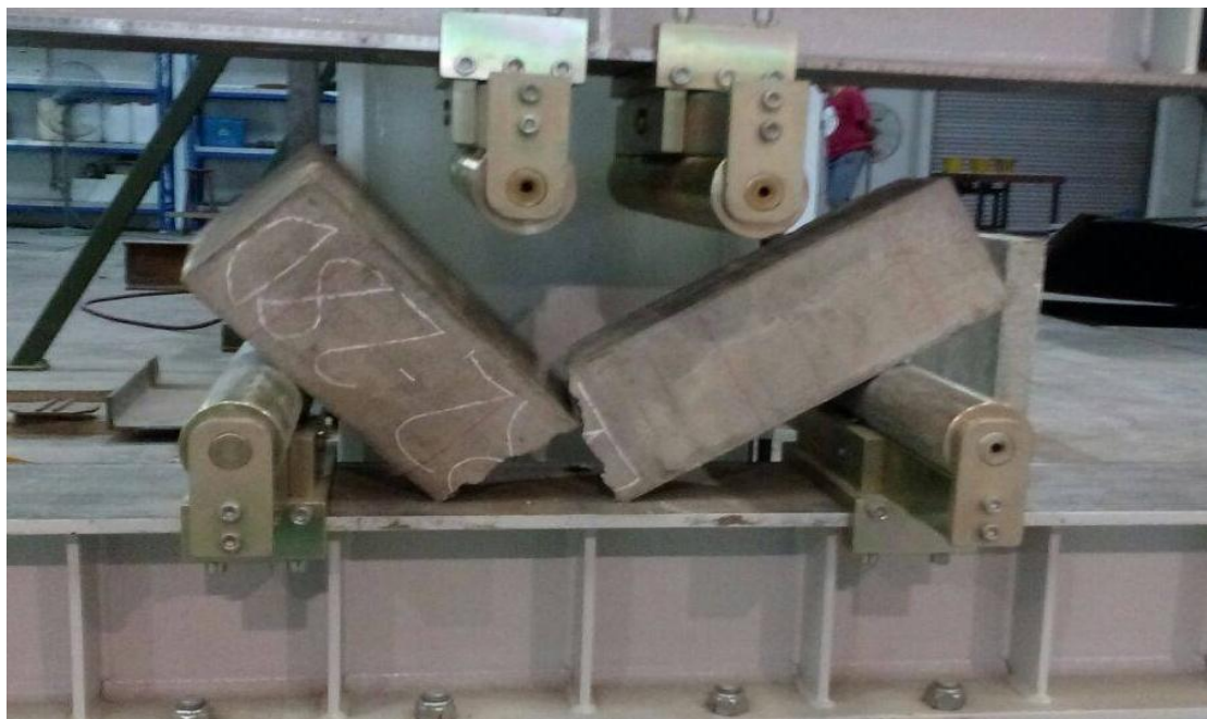
Figure 4.23: Patten of failure of beam on days 28 for ratio 2 sample
