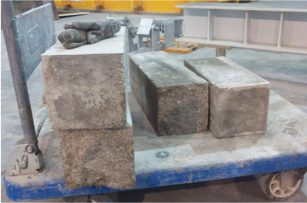
Figure 4.26: 0% of polystyrene beads in concrete for control
