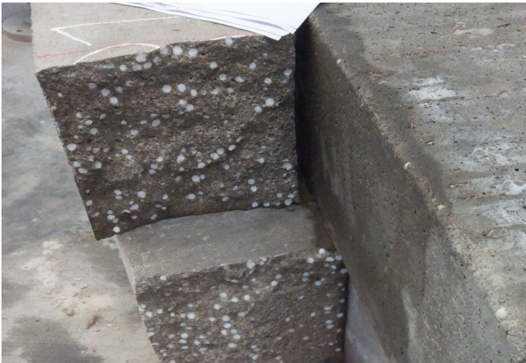
Figure 4.27: 12% of polystyrene beads in concrete for ratio 1
