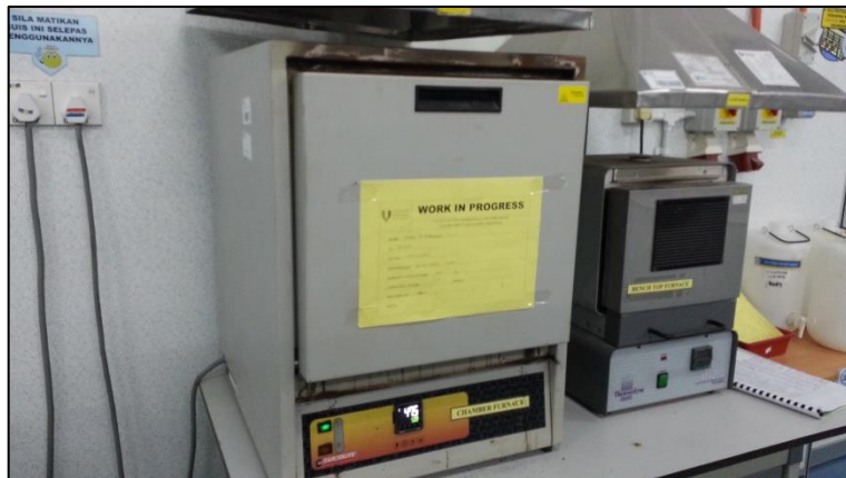
Figure 2: Burning the coconut shell at 500 °C in the furnace.
