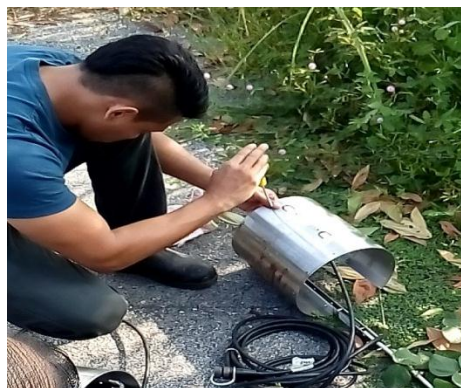
Figure 3.11: Lab assistant screws the sensor to mounting ring
