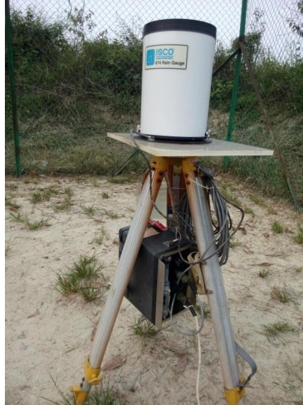
Figure 3.13: The ISCO 674 tipping bucket rain gauge installed at the free space
