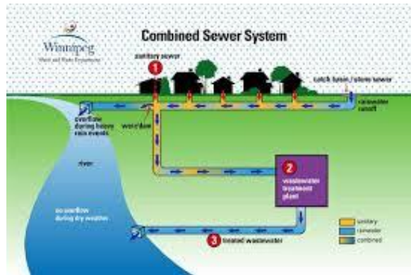
Figure 2.1: Combined sewerage system
