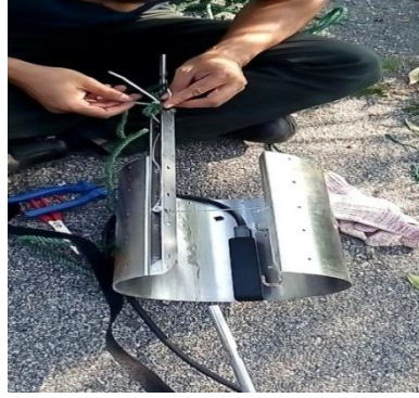
Figure 3.5: Sensor connected to mounting ring
