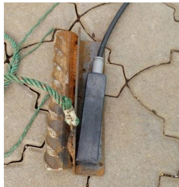
Figure 3.6: Sensor connected to steel plate and steel bar
