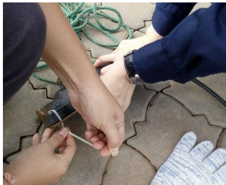
Figure 3.7: Sensor tightened at steel plate with cable tight
