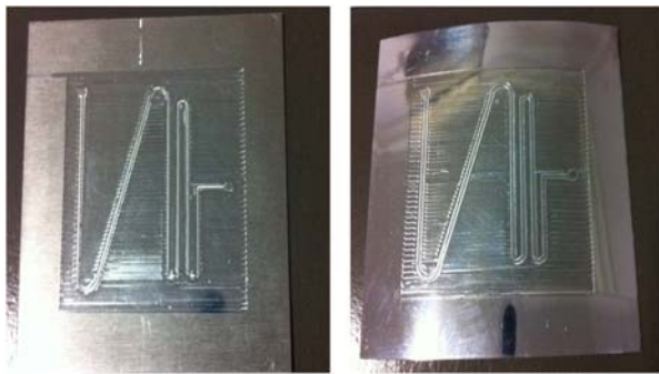
Figure-3. The 500 µm (left) and 260 µm (right) micro-milled mould.
