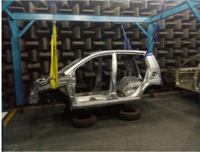
Fig. 4. Hanging BIW structure under free-free boundary condition.
