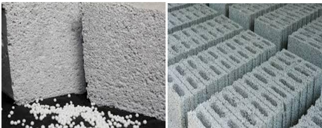
Figure 1.2: Lightweight concrete using polystyrene beads (EPS)
