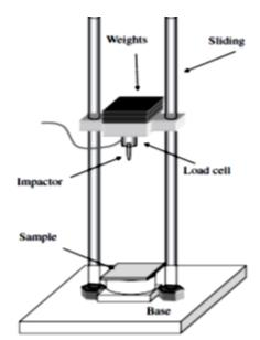
Fig 6. Drop weight impact tower [21].
