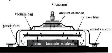
Fig 3. Schematic Representation of Vacuum bag system [14]
