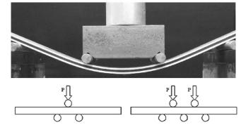
Fig 4. Photograph of a three, four and five point bending test. [13, 21]
