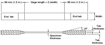
Fig 5.Tensile test specimen configuration
