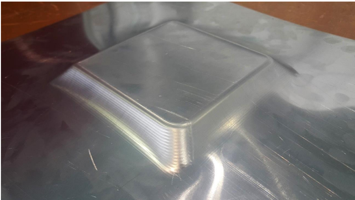
Figure 4.3: Bottom view of the aluminium sheet after ISF
