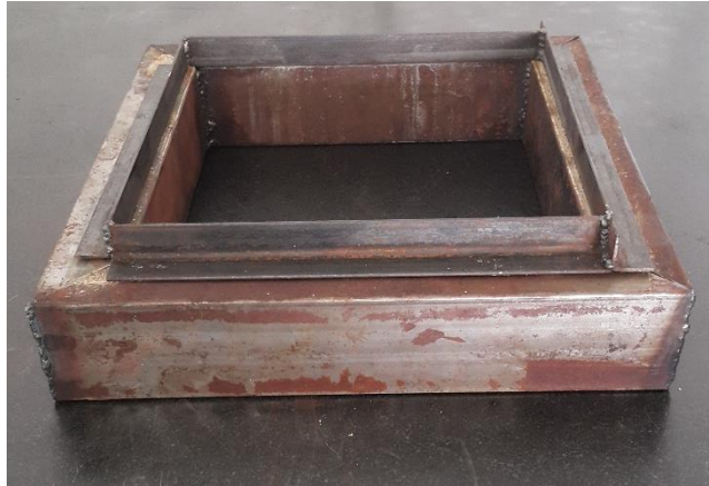
Figure 3.3: Complete structure of blank holder for ISF
