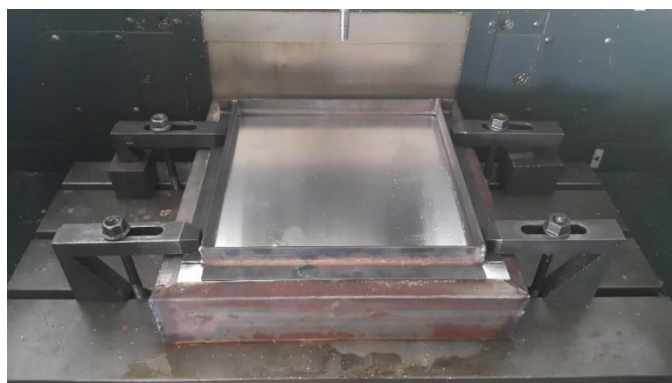
Figure 3.7: Experiment setup for ISF on CNC milling machine
