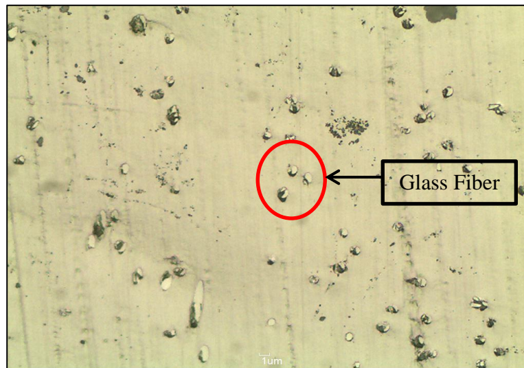
Figure 4.56 : Structure of 95%PA6 + 5%GF
