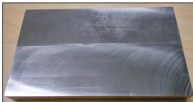
Figure 3.5: Surface finish from face milling process
