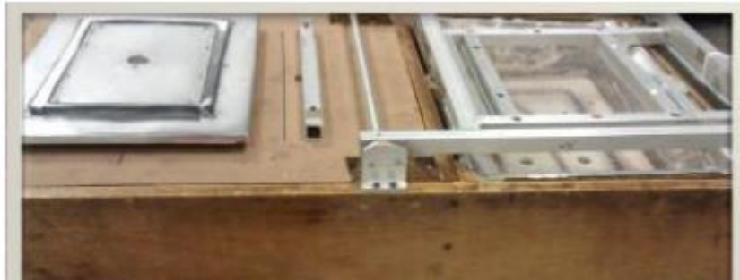
Figure 3.14. Hobby Vacuum (Drape Forming Machine)
