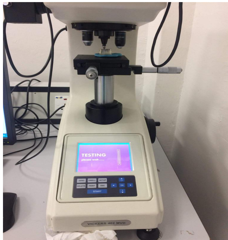
c) Vickers micro hardness testing machine
