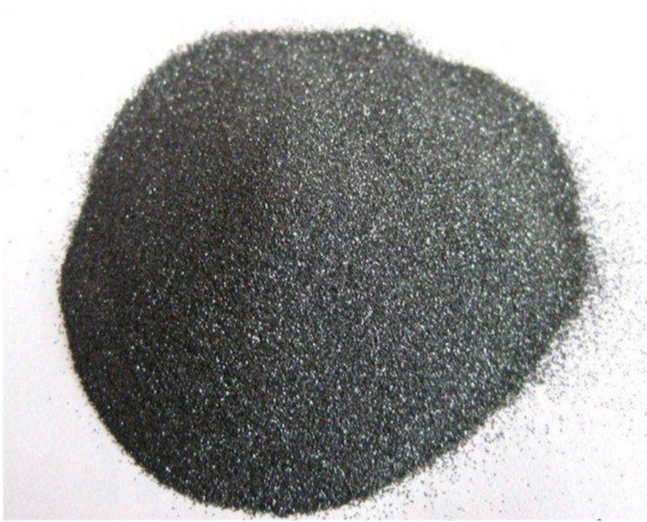
Figure 2.3: Commercially available silicon carbides particles
