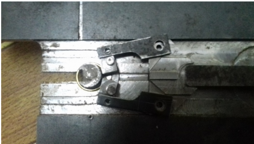
Figure 4.4: The ring forming after the bending process
