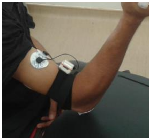
Figure 3.3: Sensor placement on biceps brachii muscle
