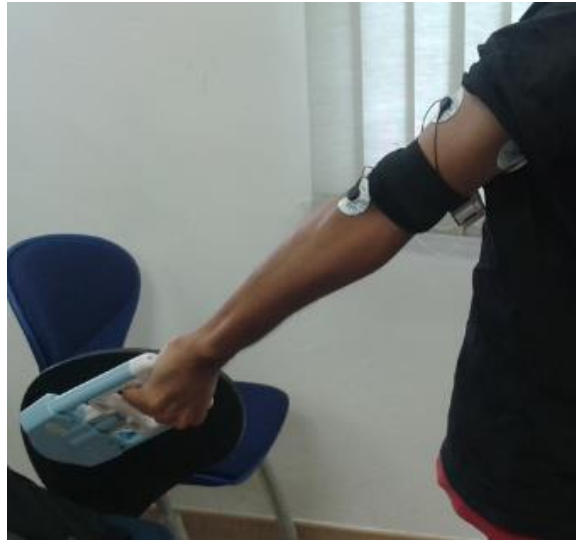
Figure 3.4: Sensor placement on triceps muscle
