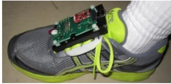
Figure 2.12: IMU secured to the shoe
