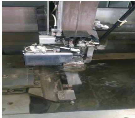
Figure 3.78: Cutting workpiece material using wire cut
