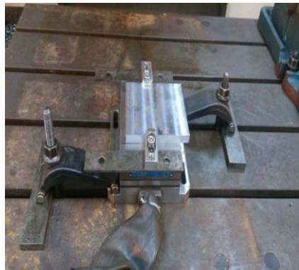
Figure 3.80: Workpiece material on dynamometer
