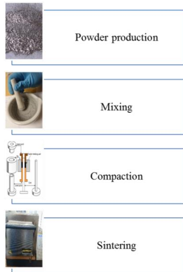
Figure 2.4: Process of Powder Metallurgy
