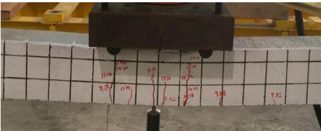
**Figure 4.18:** Flexural cracks on control beam
