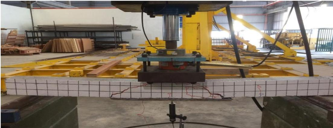
**Figure 4.19:** Overview of crack pattern on beam with PALF 1
