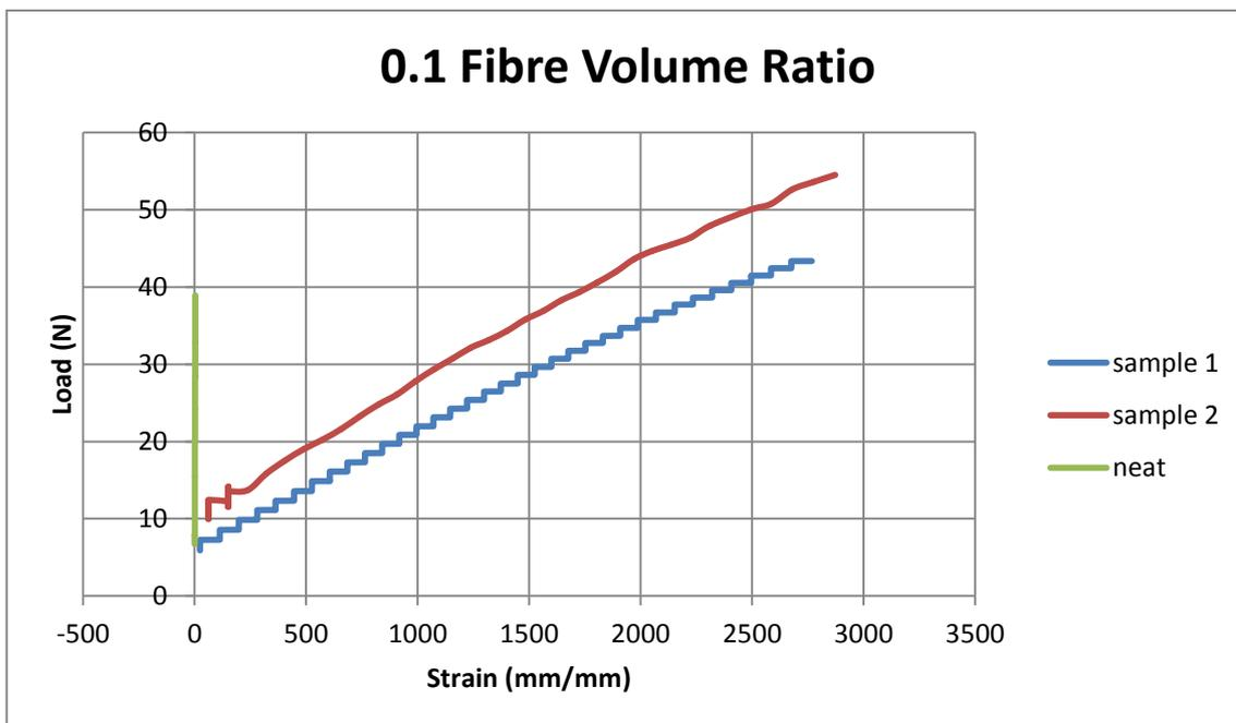
**Figure 4.7:** Load versus strain curve of composite samples with 0.1 fibre volume ratio
