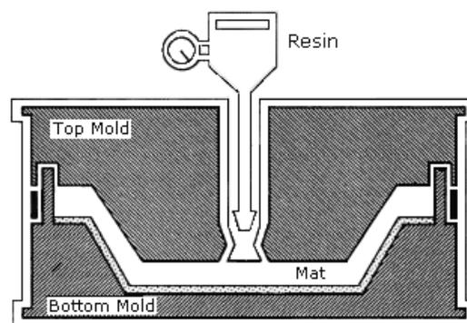
**Figure 2.4:** Resin Transfer Moulding (RTM)
