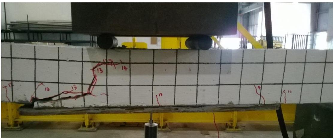
**Figure 4.22:** Diagonal shear cracks on the both end sides of the plate
