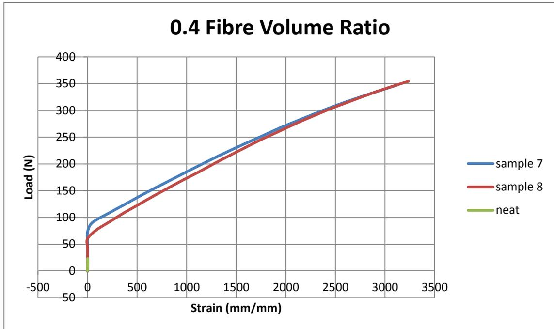
**Figure 4.10:** Load versus strain curve of composite samples with 0.4 fibre volume ratio
