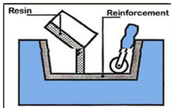
**Figure 2.5:** Hand lay-up method
