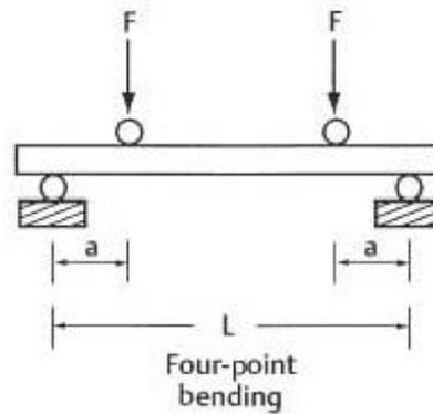
**Figure 2.18:** Four-point bending test
