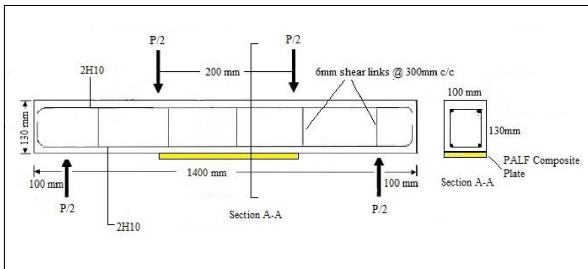
**Figure 3.21:** Schematic diagram of four-point bending test
