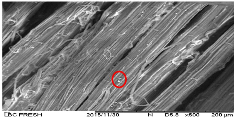
**Figure 4.1:** SEM of untreated PALF
