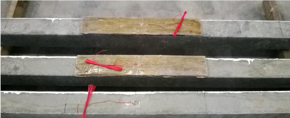
**Figure 3.22:** Composite plates together with strain gages were attached to mid-span bottom soffit of the beam
