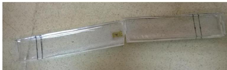
**Figure 4.12:** Neat epoxy sample after flexural test
