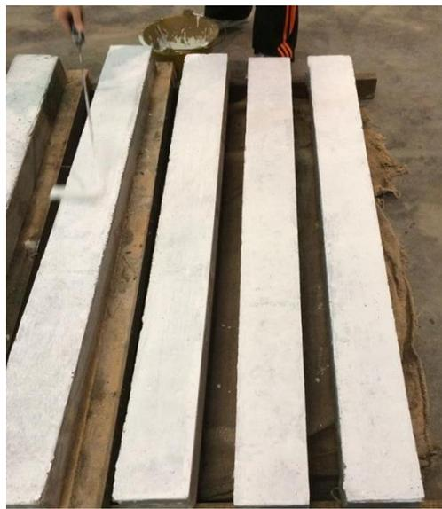
**Figure 3.17:** Beams painted with white paint
