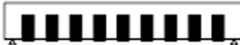
**Figure 2.15:** Strip wrapping of beam with Jute FRP
