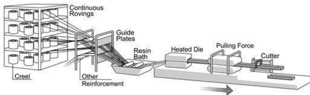
**Figure 2.2:** The pultrusion process
