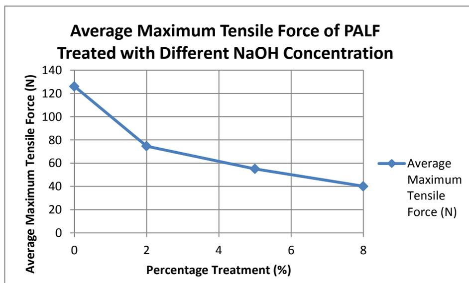
**Figure 4.5:** Average maximum tensile force of PALF treated with different concentration of NaOH
