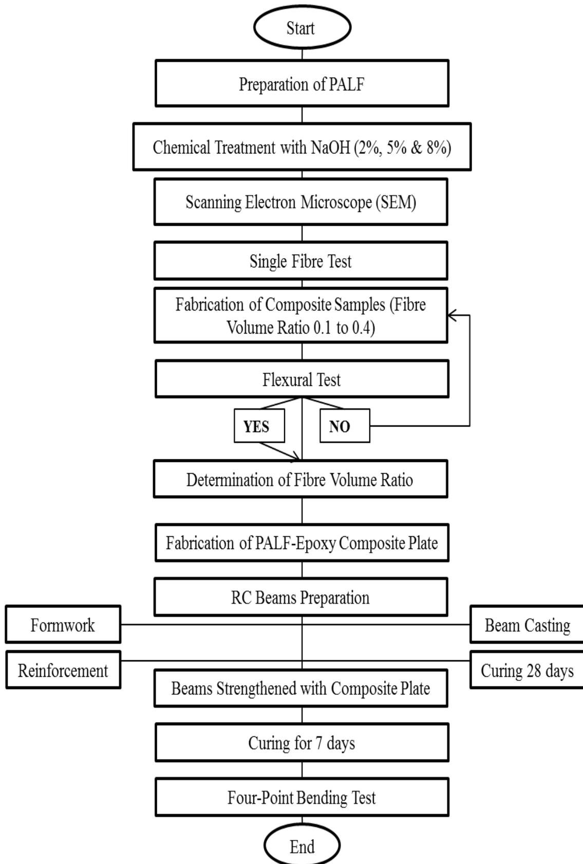
**Figure 3.1:** Experimental Work Flow of the Research
