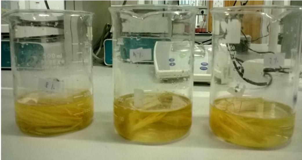
**Figure 3.6:** The fibres treated with 2%, 5% and 8% of NaOH solution (from right)
