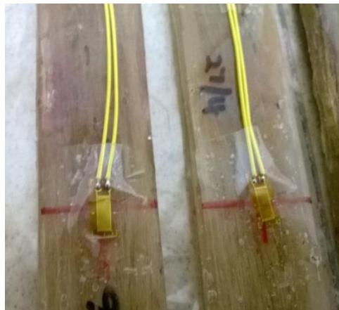
**Figure 3.20:** Strain gages were pasted at the bottom and midway of composite plate
