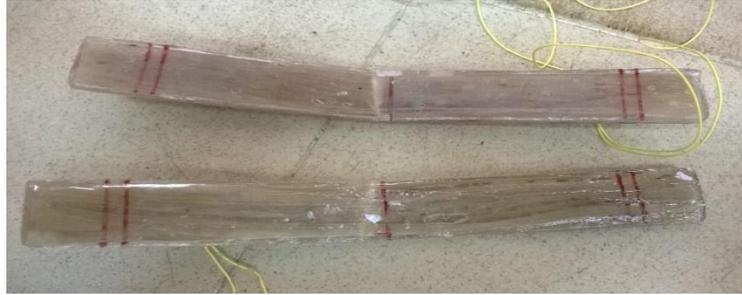
**Figure 4.13:** Top view of composite sample after flexural test
