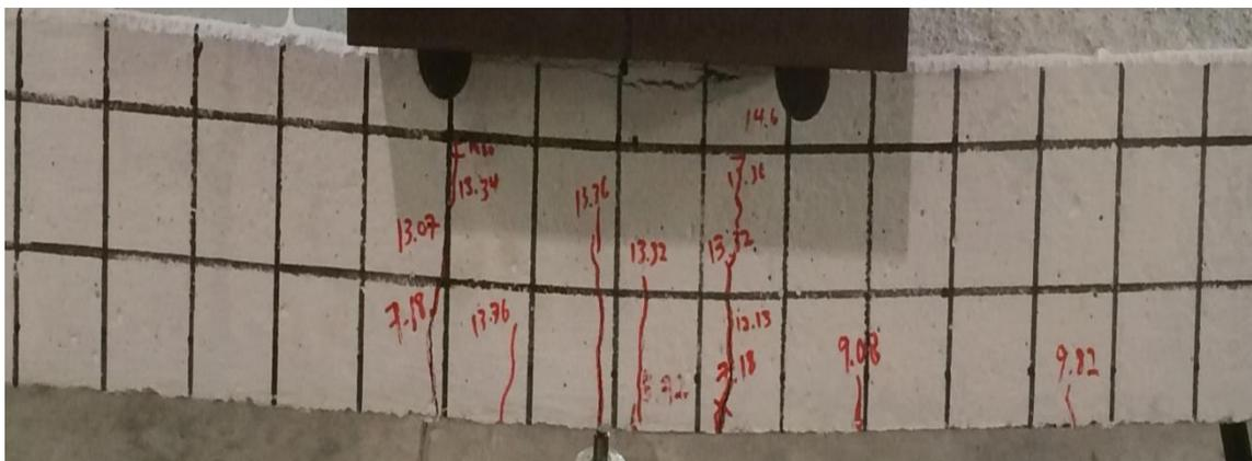
**Figure 4.23:** Failure mode of control beam
