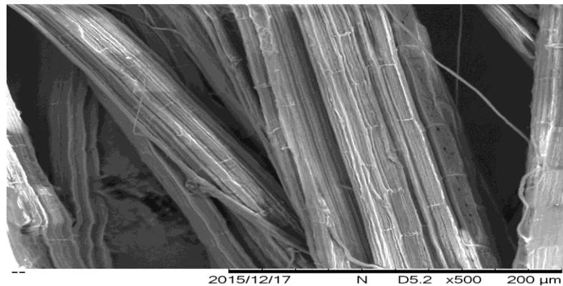
**Figure 4.2:** SEM of PALF treated with 2% of NaOH solution
