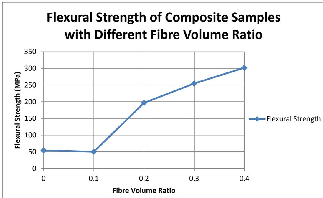
**Figure 4.11:** Flexural Strength of Composite Samples with Different Fibre Volume Ratio
