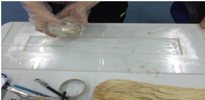
**Figure 3.10:** A layer of epoxy mixed with hardener was laid at the bottom of mould
