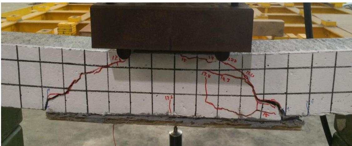
**Figure 4.20:** Shear cracks at the both end sides of the plate
