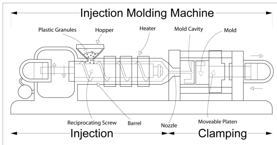
**Figure 2.3:** Injection Moulding Machine
