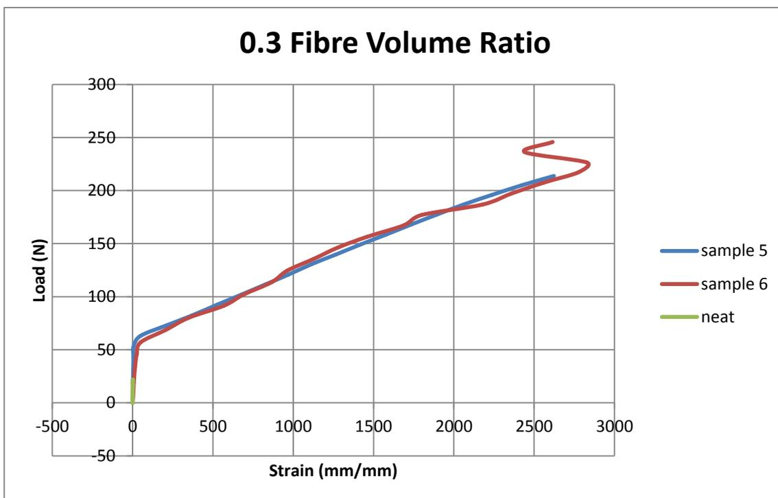
**Figure 4.9:** Load versus strain curve of composite samples with 0.3 fibre volume ratio
