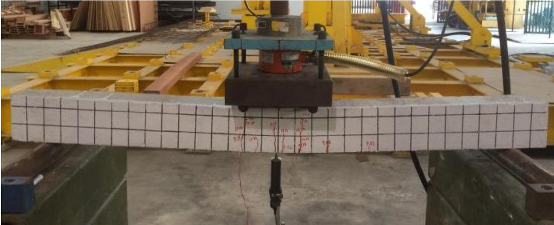
**Figure 4.17:** Overview of crack pattern on control beam
