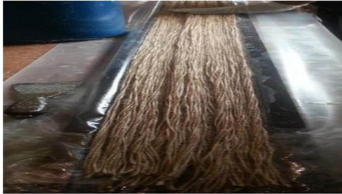
**Figure 2.11:** Jute rope composite plate
