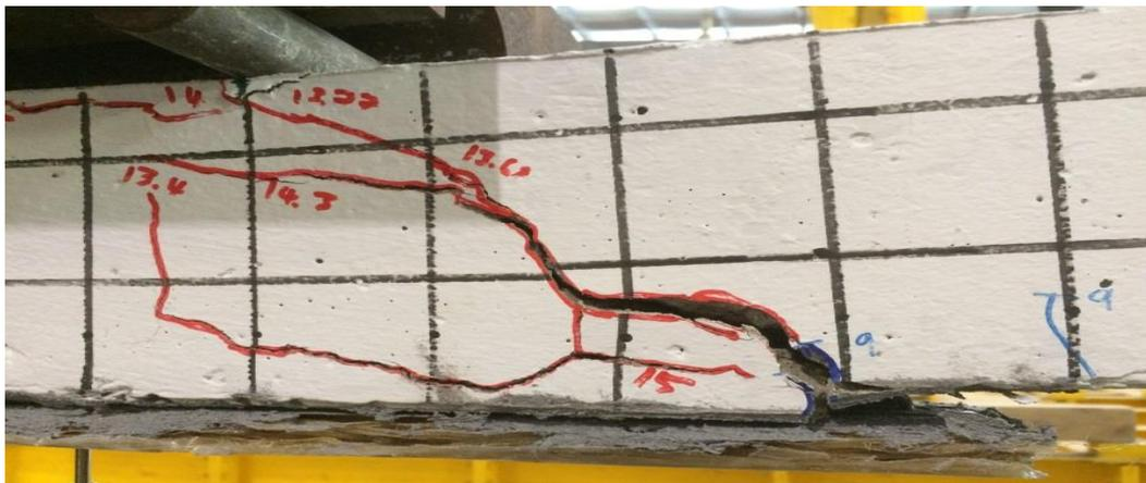
**Figure 4.24:** The plate end interfacial debonding of PALF B1
