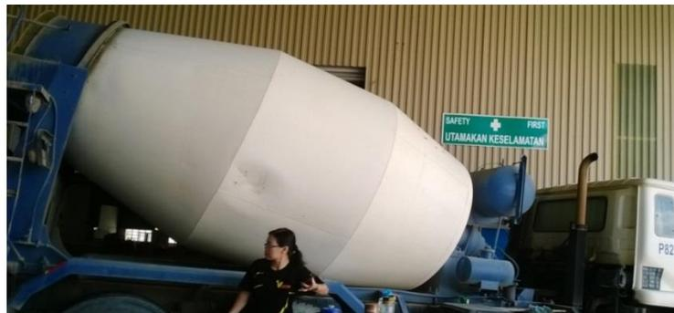
**Figure 3.15:** Fresh concrete was supplied by a concrete mixing transport truck
