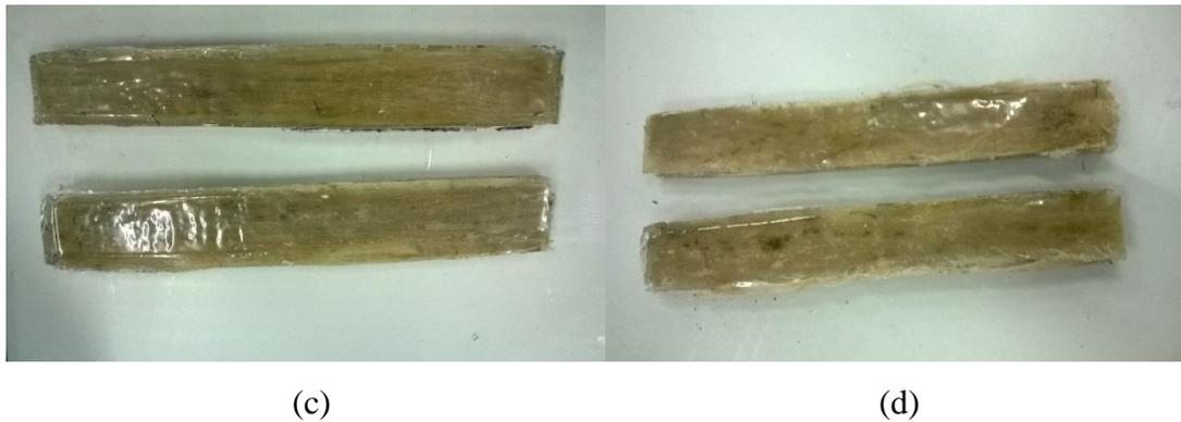
**Figure 3.8:** Composite samples with fibre volume ratio (a) 0.1; (b) 0.2; (c) 0.3; (d) 0.4
