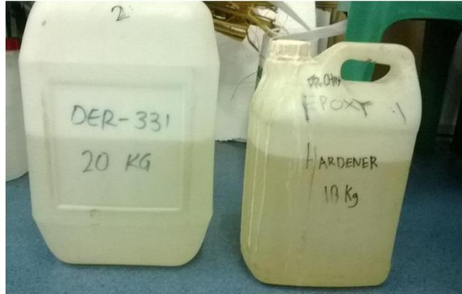
**Figure 3.3:** Epoxy DER-331 and hardener
