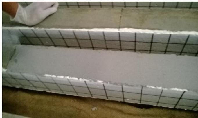
**Figure 3.4:** Concrete applied with Sikadur 30
