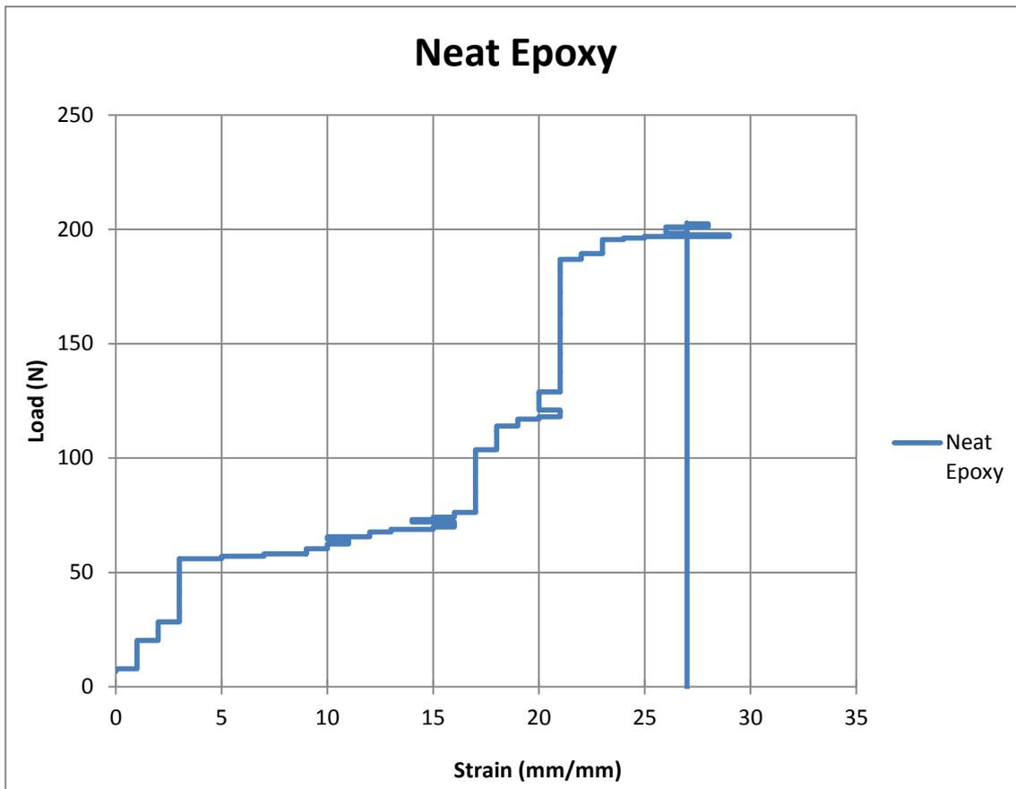
**Figure 4.6:** Load versus strain curve of neat epoxy composite samples
