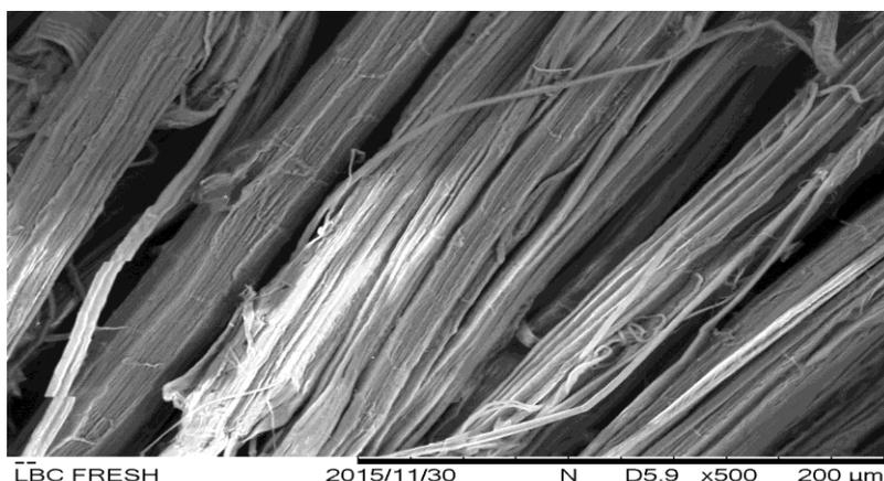
**Figure 4.4:** SEM of PALF treated with 8% NaOH solution
