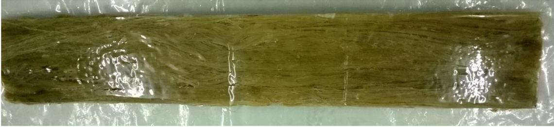
**Figure 3.12:** PALF composite plate
