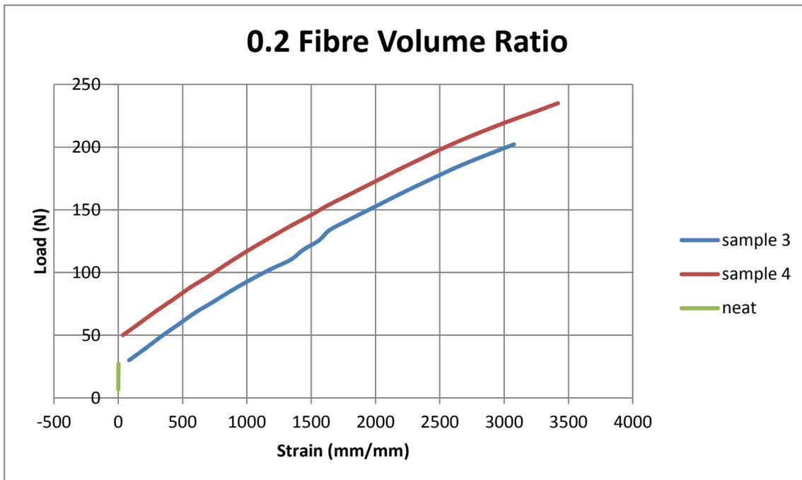
**Figure 4.8:** Load versus strain curve of composite samples with 0.2 fibre volume ratio
