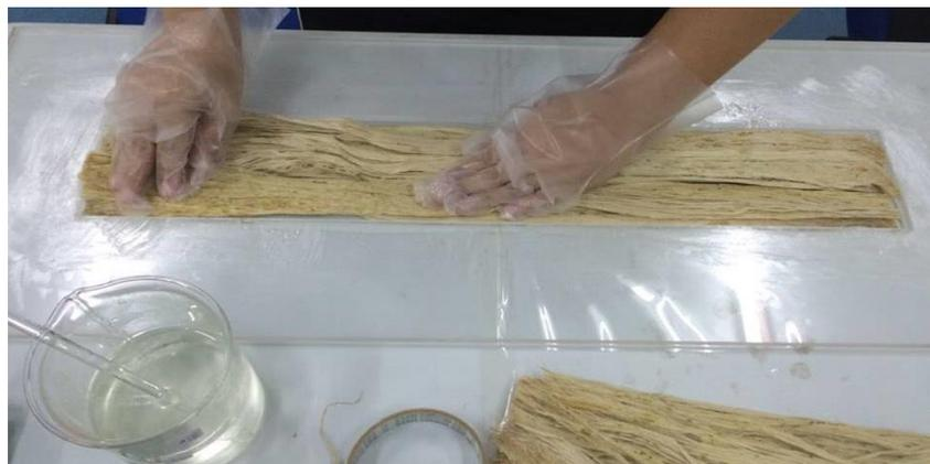
**Figure 3.11:** A layer of fibre was laid onto the epoxy adhesive
