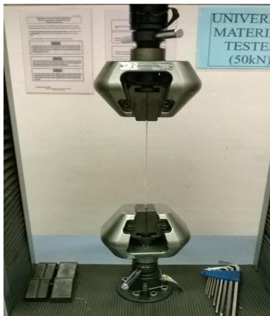
**Figure 3.18:** Single Fibre Test using UTM machine
