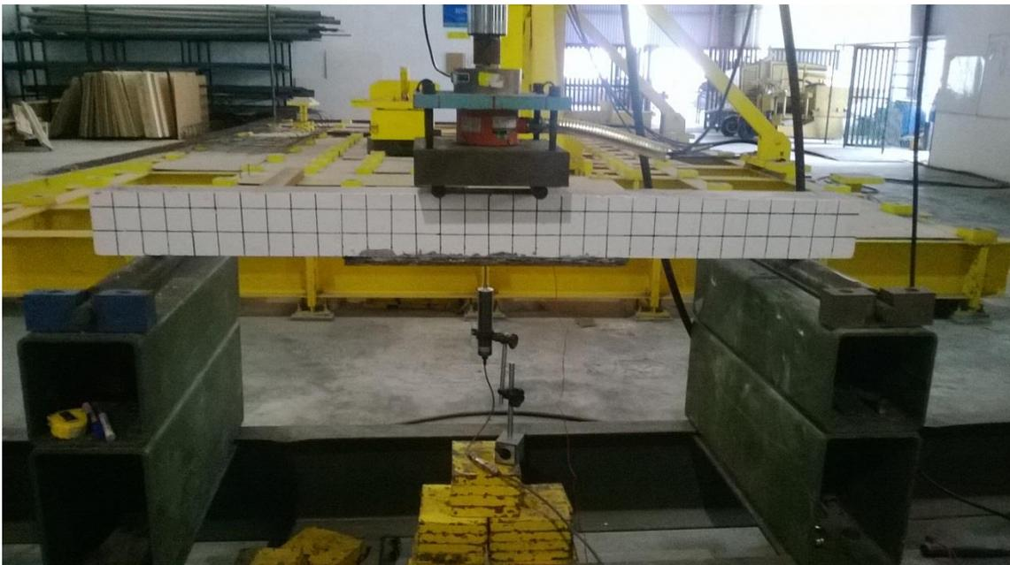
**Figure 3.23:** Four-point bending test
