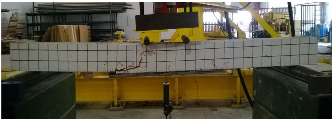
**Figure 4.21:** Overview of crack pattern on beam with PALF 2
