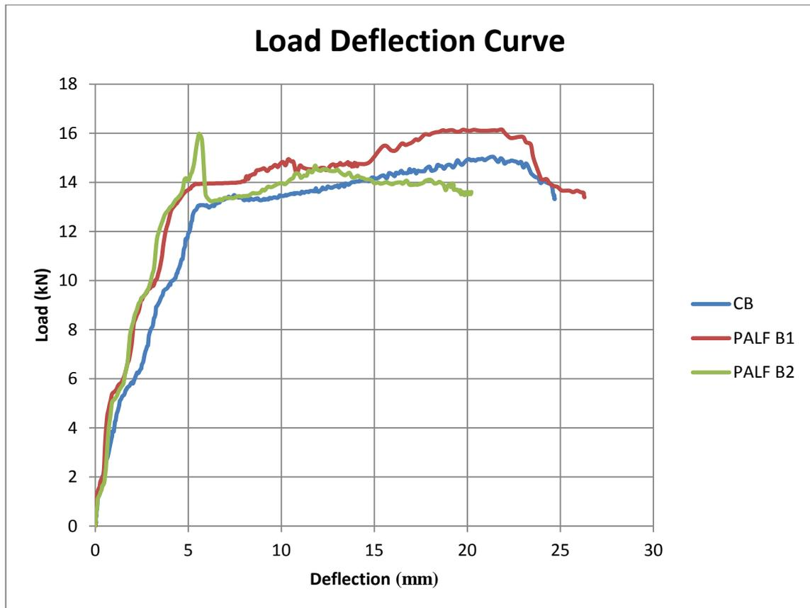
**Figure 4.16:** Load deflection curve of beam specimens
