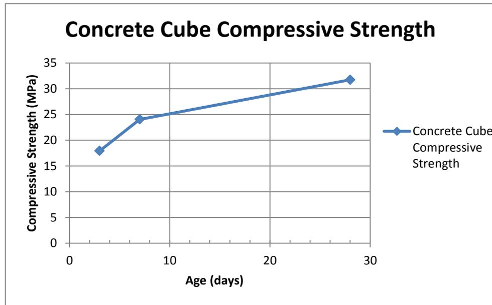
**Figure 4.15:** Compressive strength of cubes samples at 3,7 and 28 days
