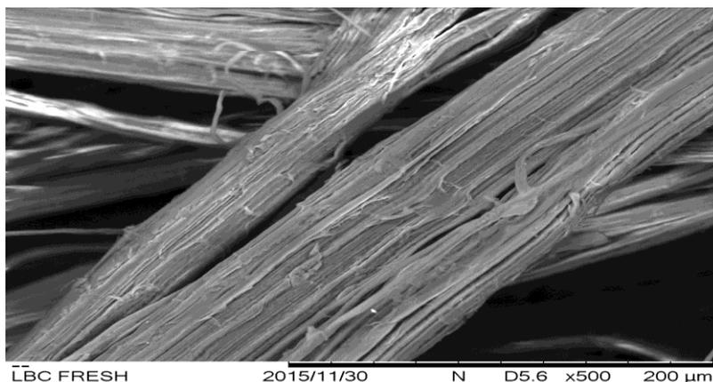
**Figure 4.3:** SEM of PALF treated with 5% of NaOH solution
