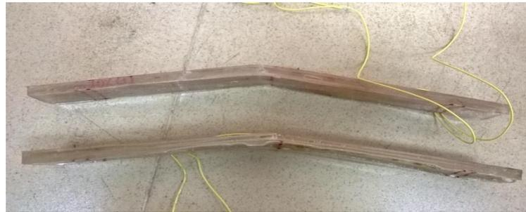
**Figure 4.14:** Side view of composite sample after flexural test
