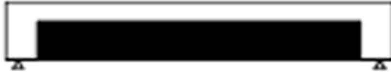
**Figure 2.14:** Full length wrapping of RC beam with Jute FRP
