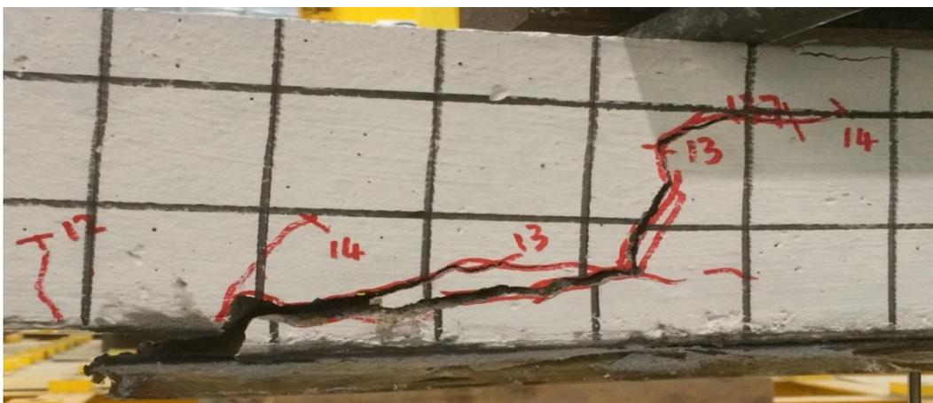
**Figure 4.25:** The plate end interfacial debonding of PALF B2
