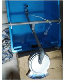
Figure 9 (b) Fig. 9. Test tank setup for thrust measurement
