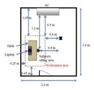
**Fig. 1.** The arrangement in environmental chamber.
