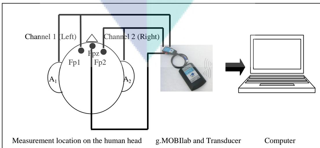
Figure 4.4: EEG Equipment Set-up
