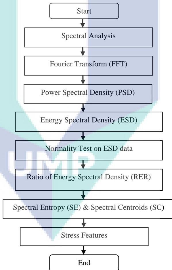
Figure 4.3: Process Flow to Identify Stress Features
