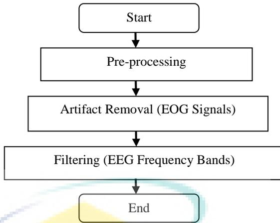
Figure 4.2: Process Flow of EEG Pre-processing
