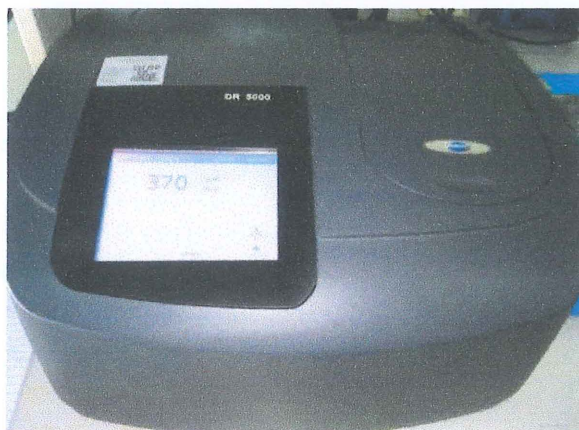
Figure 3.6: Spectrophotometer HACH DR 5000
