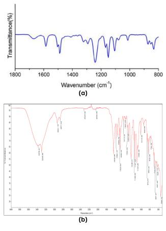
Figure 7 The spectra wavelength of the film; (a) the control data of PSf, (b) PSf/Pebax 1657 composite membranes
