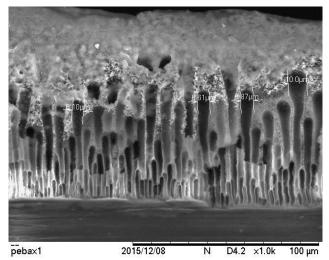
Figure 5 Cross sectional view of composite membrane with Pebax 1657 coating layer
