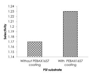
Figure 3 Selectivity for PSf substrate with and without Pebax 1657 coating
