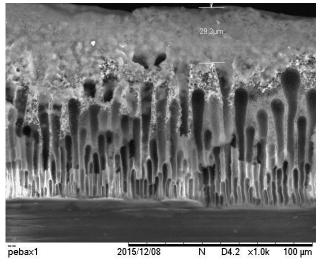
Figure 6 Thickness of composite membrane with Pebax 1657 coating layer
