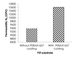
Figure 2 Permeability of  $N_2$  for PSf substrate with and without Pebax 1657 coating
