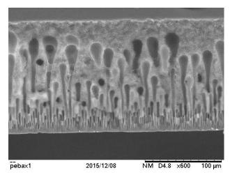
Figure 4 Cross sectional view of Psf substrate without coating
