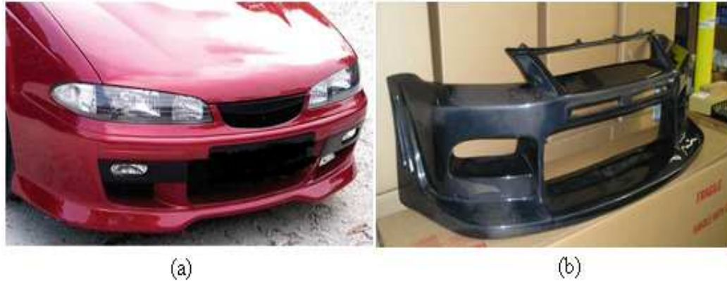
Figure 1.1 Car bumpers (a) using polyurethane (PU) material (b) using carbon-fiber reinforced polymers (CFRP) material
