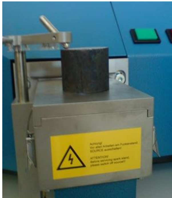
Figure 3.12: Specimen position during spark
