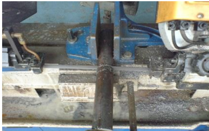
Figure 3.2: Cutting using band saw machine
