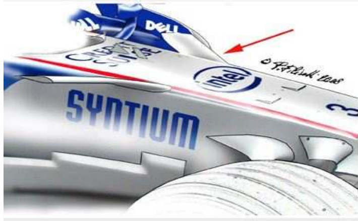
Figure 2.2: Winglets of Formula One car.
