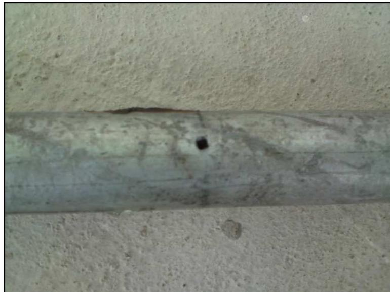
**Figure 3.2:** Hole as the source of the leak
