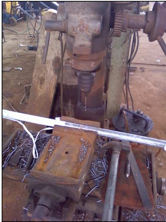
Figure 3.1: Drilled hole using drilling machine
