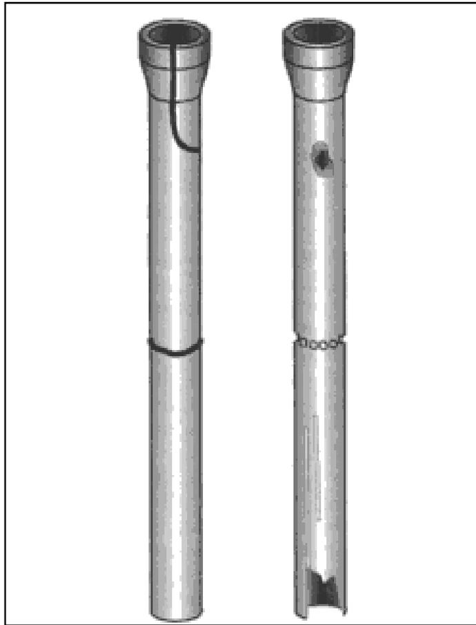
**Figure 2.1:** Failure modes for small (<380 mm) diameter pipe
