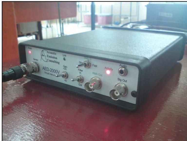
**Figure 3.9:** AED-2000V Virtual Instrument
