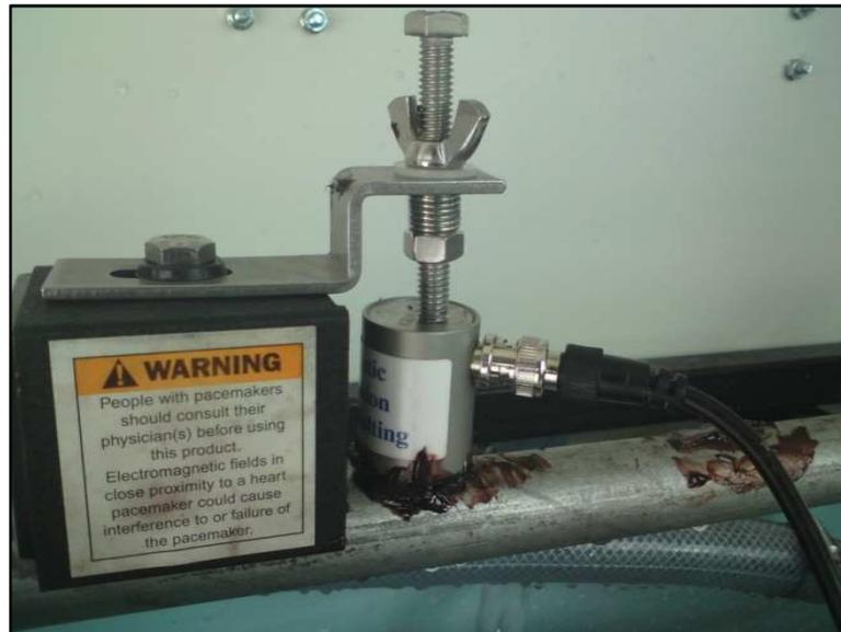
**Figure 3.8:** AE sensor
