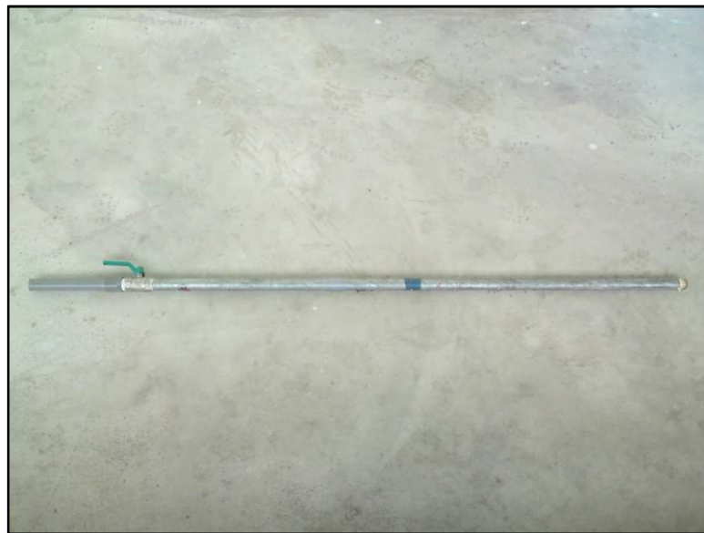
Figure 3.4: Galvanized steel pipe, \frac{3}{4} inches of diameter and 1 meter long
