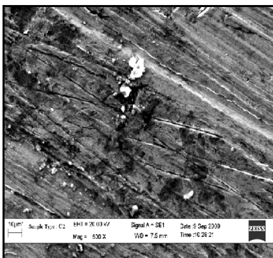
Figure 4.2: Copper surface microstructure exposed to the indoor environment
