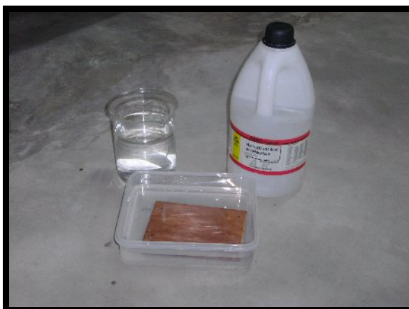
Figure 3.10: Cleaning Process using Hydrochloric Acid.
