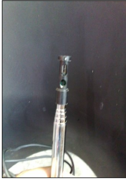
Figure 4.4: Sensor to measure temperature and velocity
