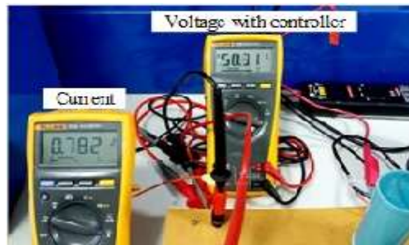
Figure 6 Experimental output values in rms with resistive loads ( R_1+R_2 )
