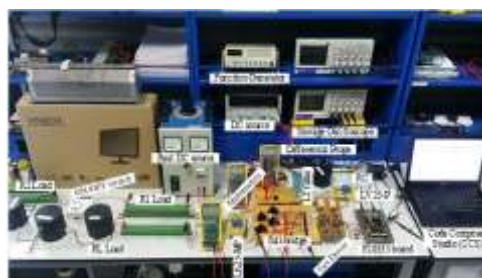
Figure 3. Hardware setup of voltage source inverter
