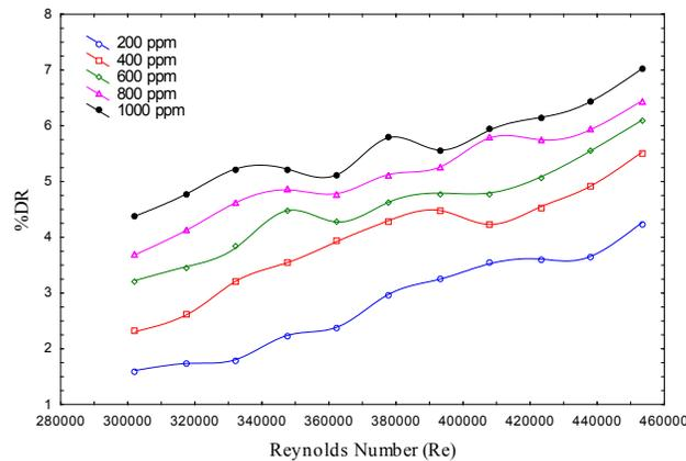
**Figure 5.** Effects of SLES Concentrations on DR Performance for Different Re Using SV-groove with H 900 μm.
