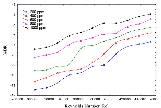
**Figure 6.** Effects of SLES Concentrations on DR Performance for Different Re Using SV-groove with H= 3100 μm.
