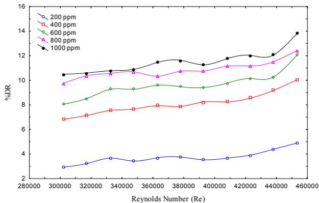
**Figure 4.** Effects of SLES Concentrations on DR Performance for Different Re Using Smooth Disk.
