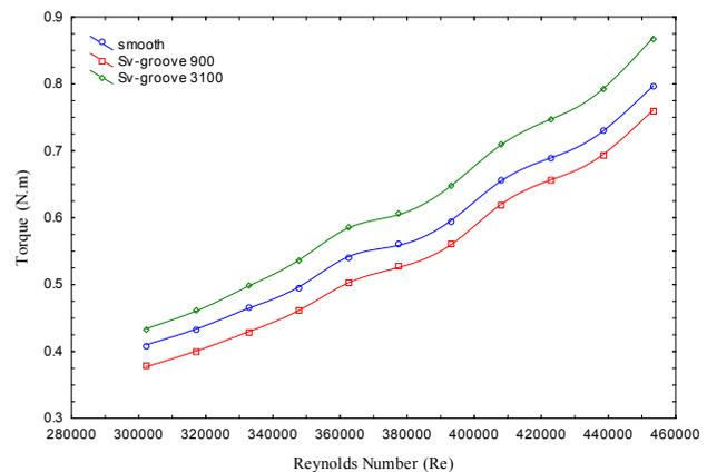
Figure 2. Effects of Re on Torque Values of Three Disk Types.
