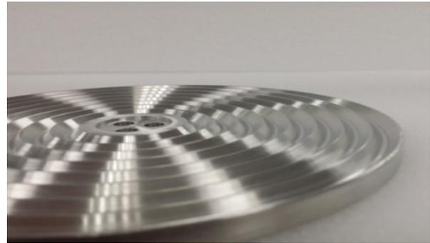
Figure 1. Photograph Pictures of SV-groove Disk.
