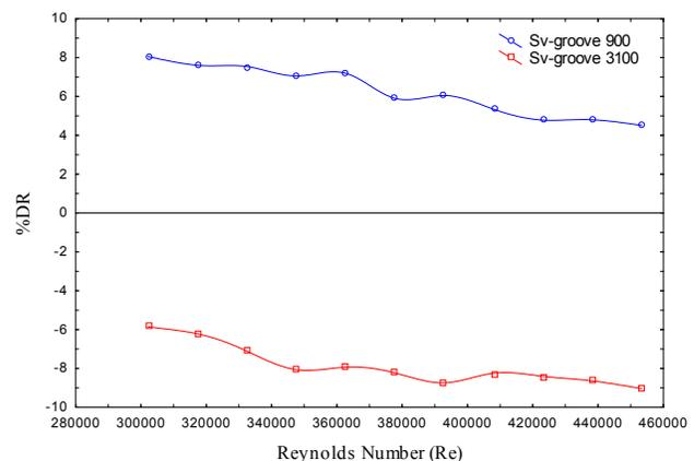
Figure 3. Effects of Re on DR Performance of SV-groove with  $H=900$  and  $3100\ \mu\text{m}$ .
