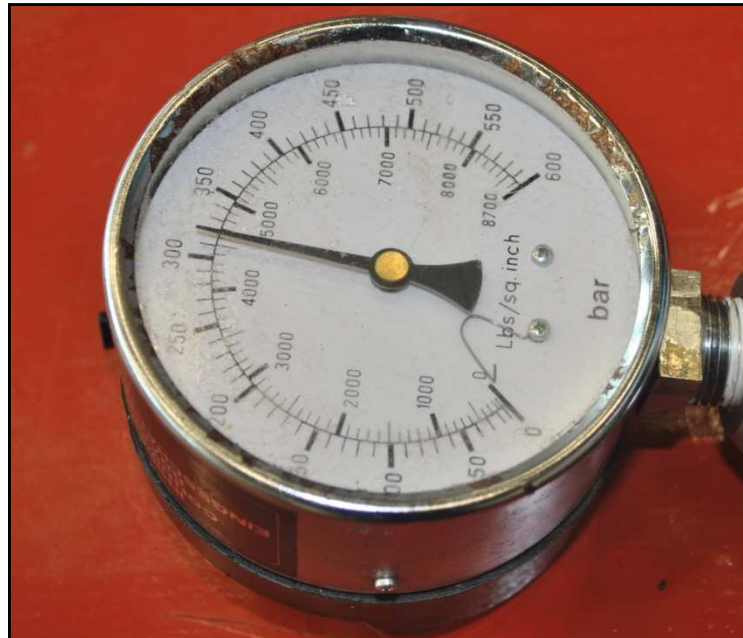
Figure 3.8: Pressure gauge for controlling pressure of injector
