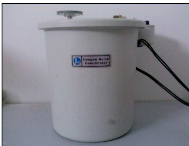
Figure 3.7: Bomb calorimeter to measure specific heat capacity
