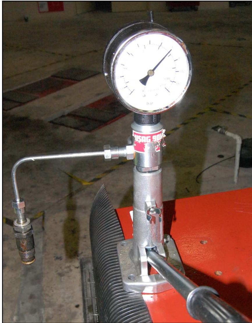
Figure 3.11: Injector tester to define the spray pattern
