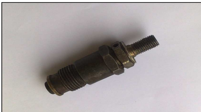
Figure 3.10: Injector of ISUZU 4x4 to produce spray pattern
