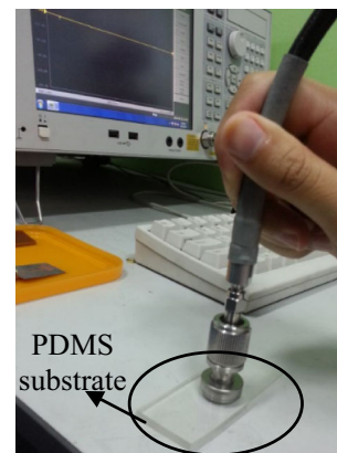
Fig. 3 Sample of PDMS substrate during permittivity measurement
