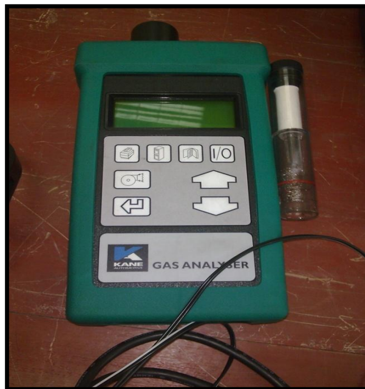
Figure 3.7 : Gas Analyzer used to measure the quantity of CO 2 , NO x , O 2 , and HC emissions in exhaust gas
