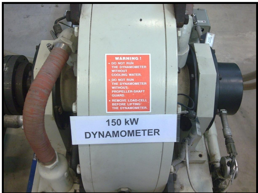
Figure 3.2 : 150 kW Eddy current Dynamometer for this engine testing
