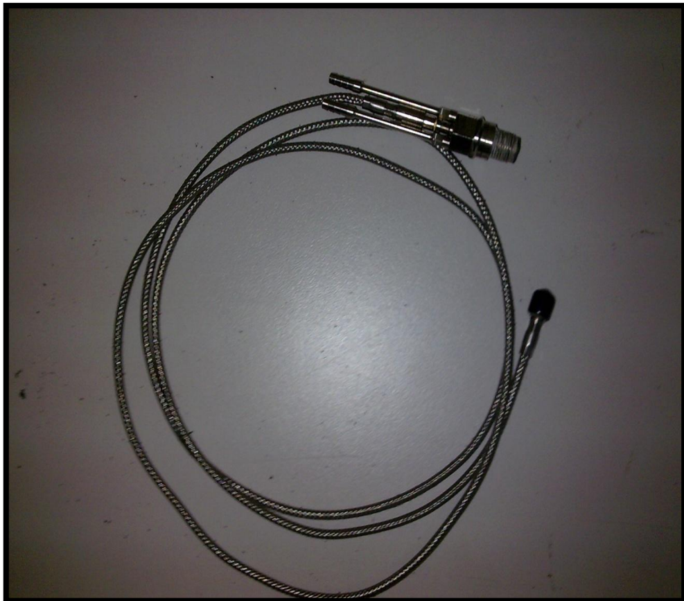
Figure 3.5 : Pressure sensor to measure in-cylinder pressure for experimental diesel engine
