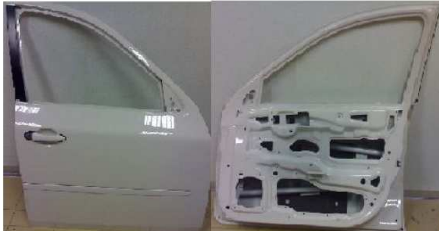
Figure 3.2: Inner and outer of door panel
