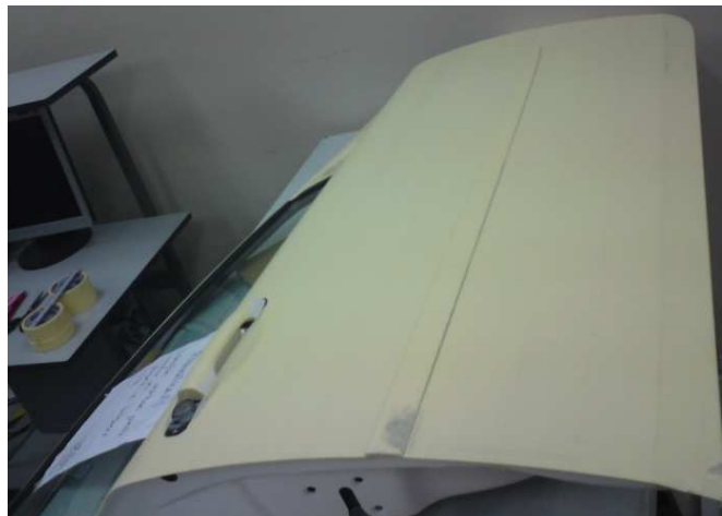
Figure 3.7: Process cover the door panel surface with masking tape
