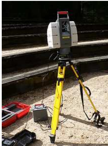
Figure 2.3: Example of 3D scanner using time of flight
