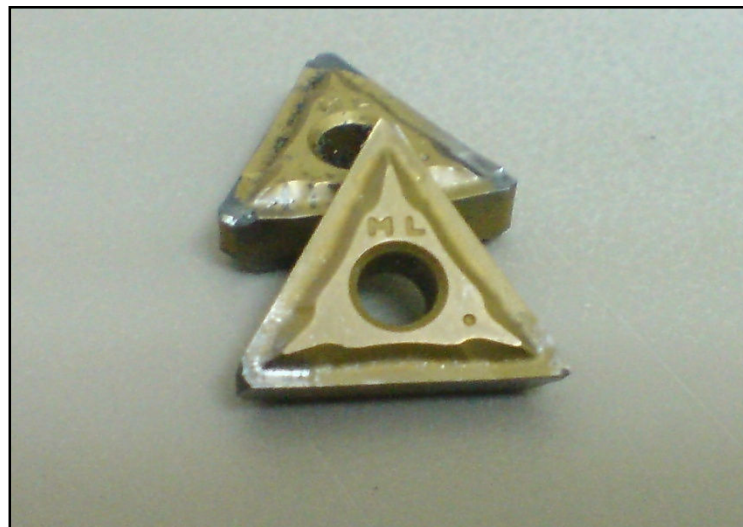
Figure 3.3: Triangle shape CVD Coated Carbide Tips inserts for lathe machine.
