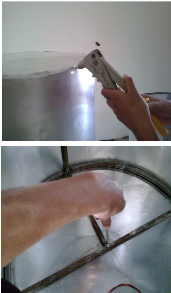
Figure 3.14: Rivets, bolts and nuts used to join the cover, main body and door
