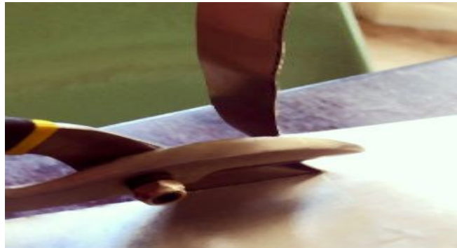
Figure 3.12: Cutting the aluminum plate with the tin snips
