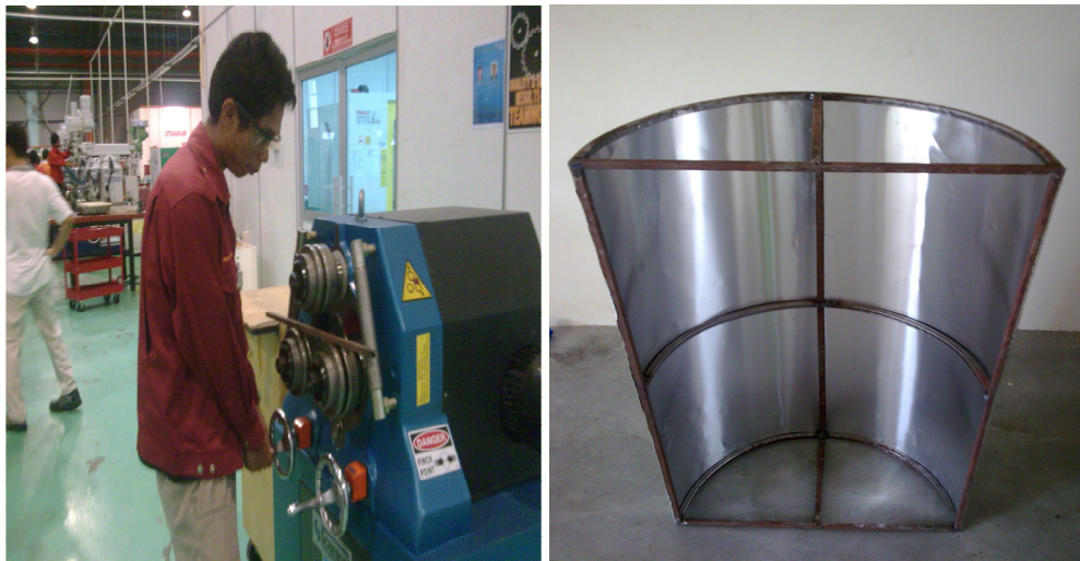
Figure 3.9: Bend the hollow steel to making the cover support
