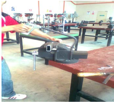
Figure 3.1: Cutting hollow stainless steel using steel saw.
